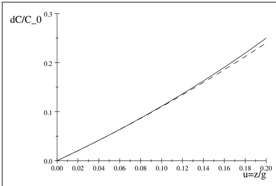
Figure 4: Plot of  $\frac{\Delta C}{C_0}$  as function of  $u = z/g$  (solid line) and the Taylor expansion (dashed line) for small values of  $u$ . Note the linear region.
