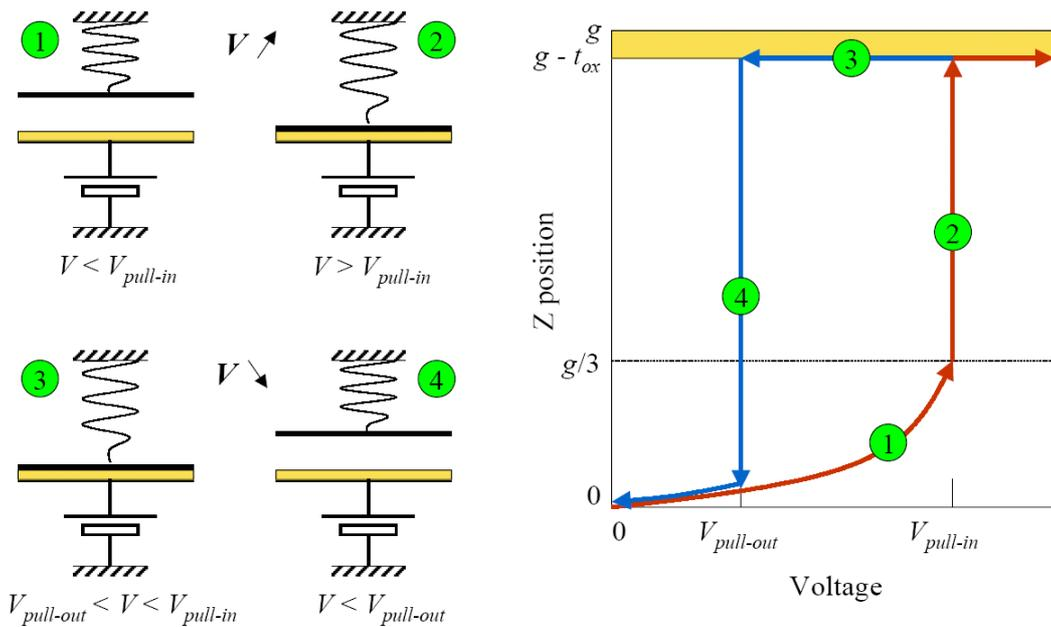
Figure 9: The system shows a hysteresis behavior depending on the voltages applied.
