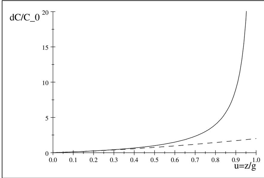
Figure 3: Plot of  $\frac{\Delta C}{C_0}$  as function of  $u = z/g$  (Eq. 12, solid line) and the Taylor expansion (Eq. 13, dashed line).
