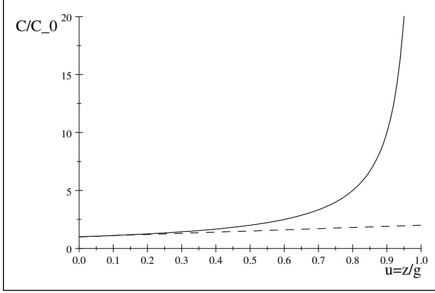
Figure 2: Plot of  $\frac{C}{C_0}$  as function of  $u = z/g$  (Eq. [8](#), solid line) and the Taylor expansion (Eq. [10](#), dashed line).
