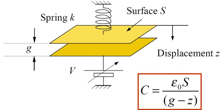
Figure 1: A capacitor with a moving plate. The initial gap is  $g$  and the spring has spring constant  $k$ .
