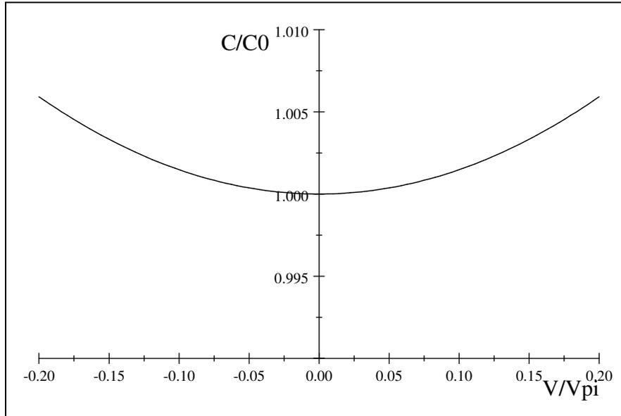
The CV curve is a parabola.
