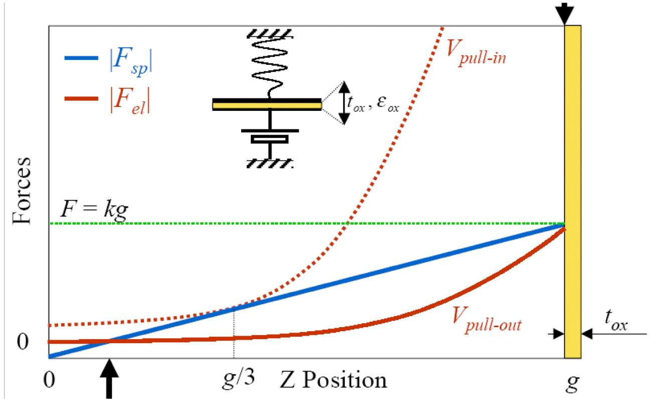
Figure 8: At pull in the moving plate touches the fixed plate and the distance between the two plates is the thickness of the oxide used as an insulation layer.
