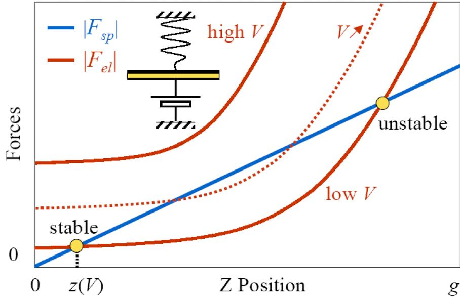
Figure 5: Plot of the spring force,  $F_{sp}$ , and the electrostatic force,  $F_{el}$ , between the plates. At high voltages the electrostatic force is always larger than the spring force and the moving plate is pulled down to the fixed plate. At lower voltages there is a stable position where the electrostatic force equals the spring force.
