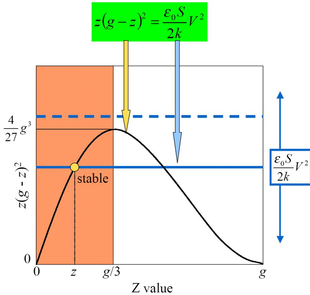
Figure 7: Plot of Eq. 28. The maximum occurs at  $z = g/3$  and below this value a stable condition is obtained.
