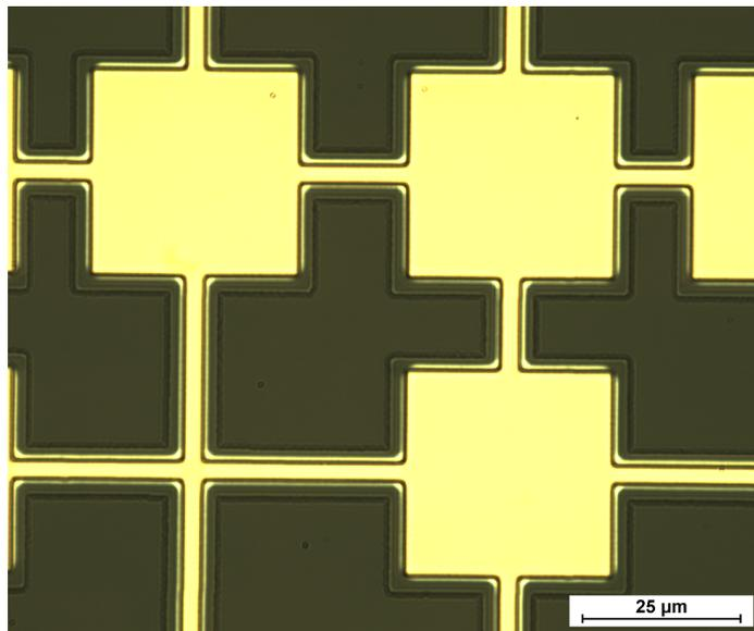
**Figure 8.4:** Microscope image of the *Bottom electrode* resist mask in the CMUT glass cavities on top of the Au electrode layer after IBE etching. The Au electrodes are now confined to the glass cavities. A halo effect likely caused by re-deposition is visible along the resist mask edge.
