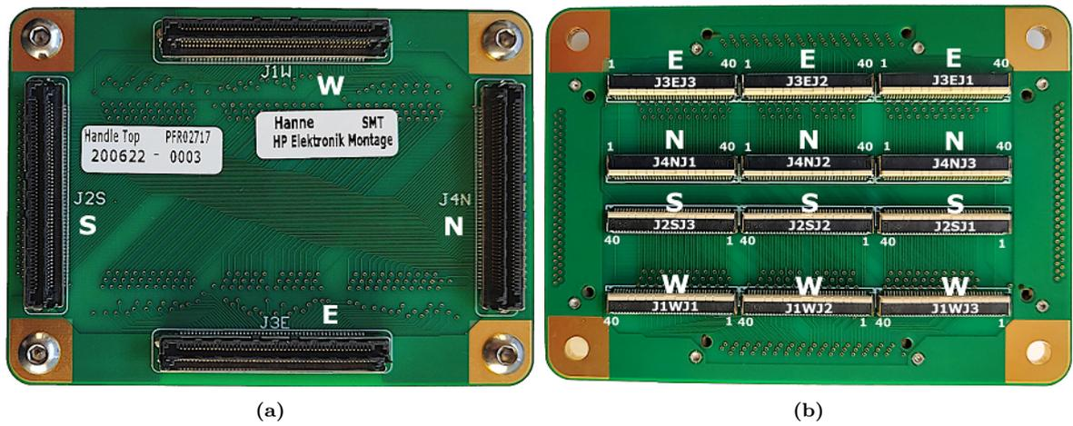
**Figure 9.29:** (a) Interposer board seen from the front with sockets for connecting the the CCB and (b) the same board seen from the back with sockets for connecting flex cables to the TABLA V preamplifier boards.
