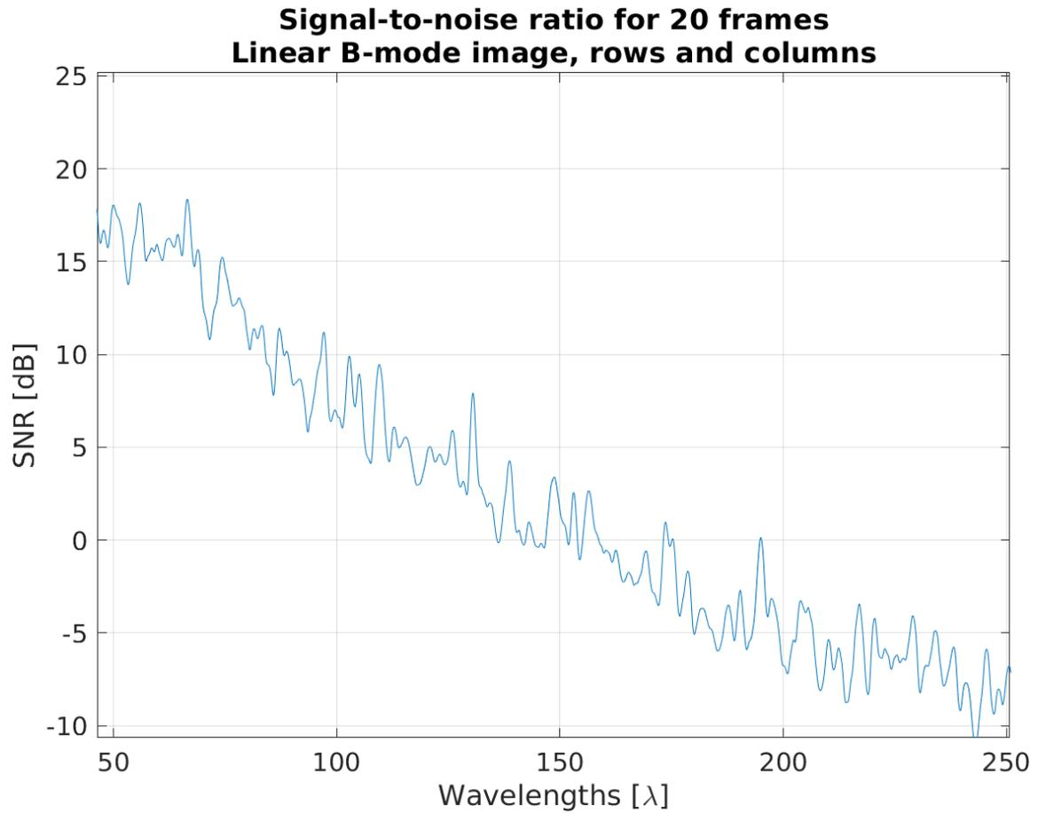
**Figure 6.39:** SNR of the 190+190 RCA probe for a tissue mimicking phantom with an acoustic attenuation of 0.5 dB/[MHz cm]. The penetration depth is roughly  $150 \lambda$  when the SNR reaches 0, corresponding to 3.6 cm as the wavelength in this phantom is 0.2375 mm when imaging with a frequency of 6.5 MHz. From [1].
