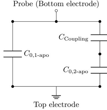
**Figure 9.40:** Circuit diagram of the neighbouring element coupling when probing column element 1, with  $C = C_{0,1-apo}$  and the signal on the bottom electrode pad and ground on the top electrode. The measured parasitic capacitance  $C_{Coupling}$  as well as  $C_{0,2-apo}$ , from the neighbouring element 2, couples into the probed element.
