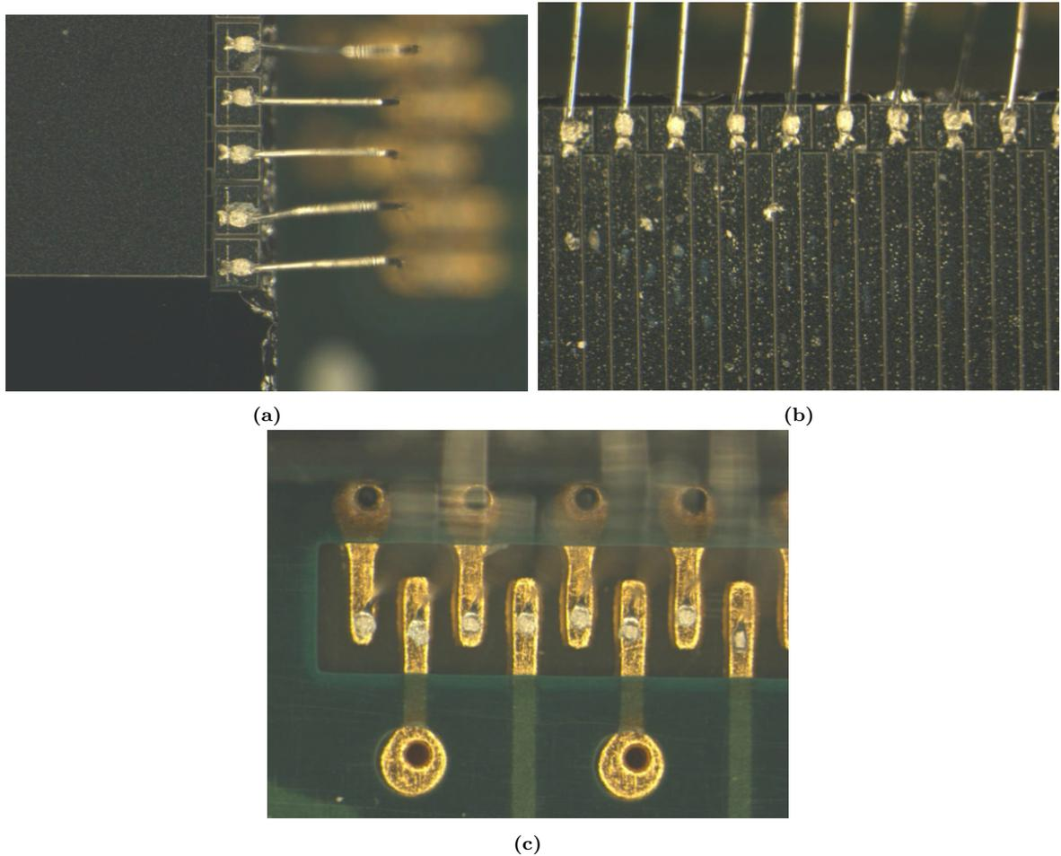
**Figure 6.8:** Close-up photos of the wedge wire bonding performed on contact pads of the columns (a) and of the rows (b) as well as on the PCB. None of the severely damaged contact pads with wire bonds have been documented.
