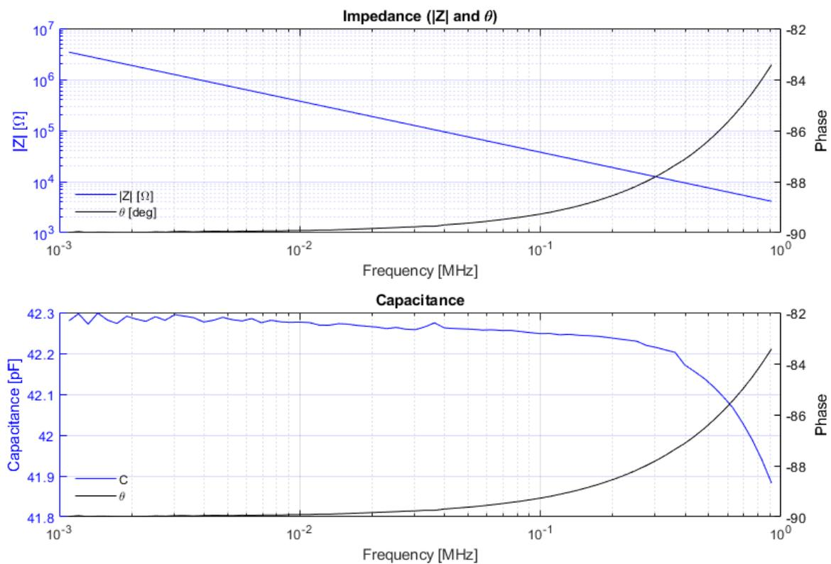
**Figure 3.5:** Plot of a typical Z-f impedance measurement on the B1500A. The magnitude of the impedance  $|Z|$  in [ $\Omega$ ], the derived capacitance  $C$  in [pF] and the phase angle  $\theta$  in [ $^\circ$ ] are plotted versus frequency from 1 kHz to 1 MHz. The capacitance versus frequency (C-f) can be used to find the optimal frequency for sweeping the capacitance versus voltage (CV).
