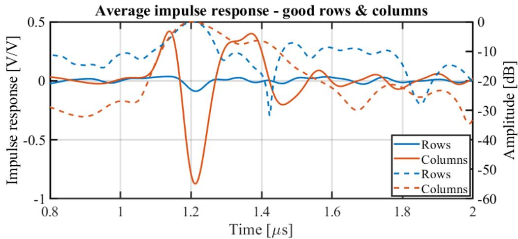
**Figure 9.35:** Average pulse-echo impulse response in transmit (PE), as solid lines, and the normalised envelope (in dB), as dashed lines, of the functional row and column elements with amplitudes above  $0.11 \times 10^{15} \text{ V V}^{-1}$  for rows and above  $0.50 \times 10^{15} \text{ V V}^{-1}$  for columns.
