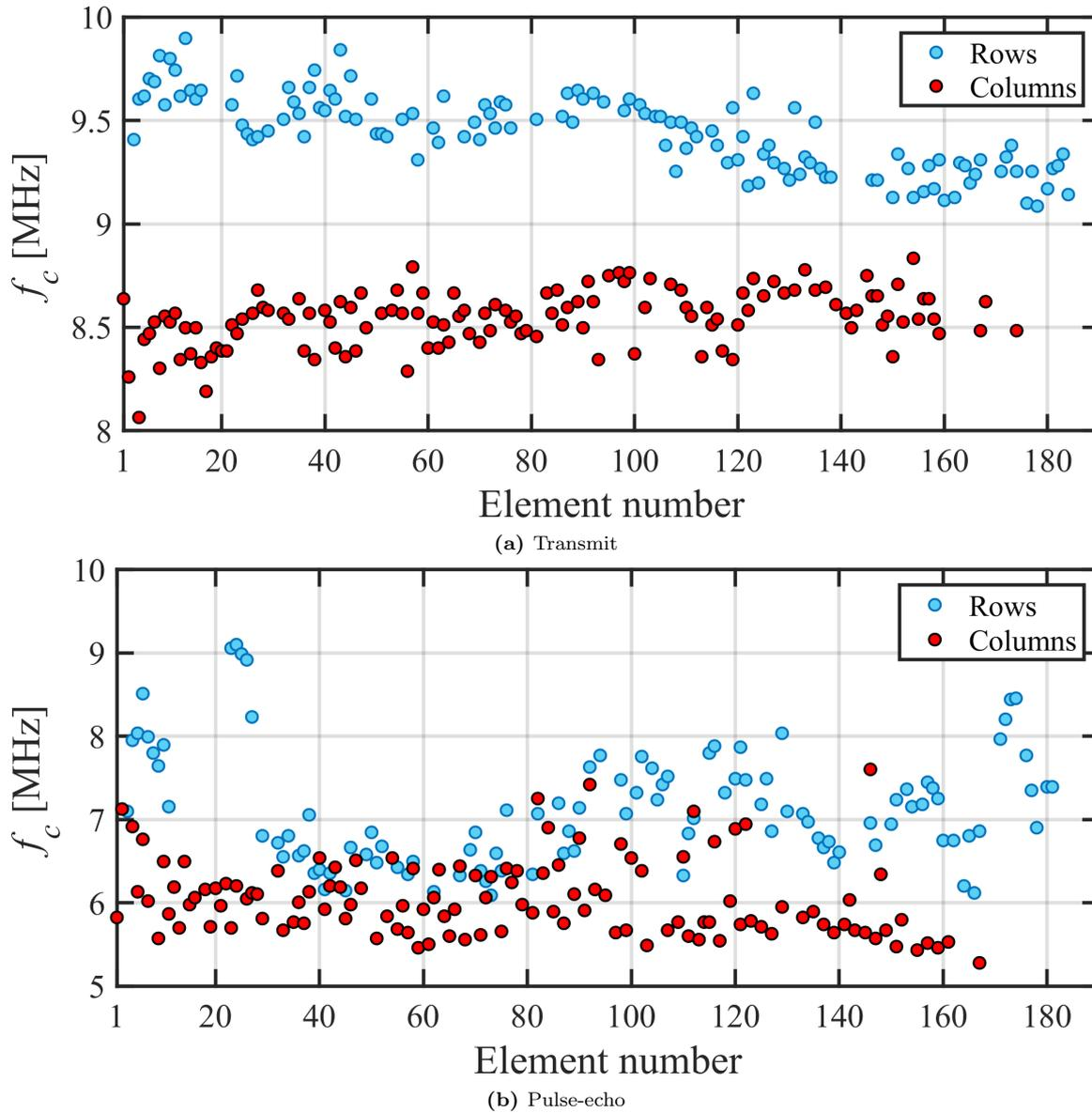
**Figure 9.38:** Extracted center frequencies across the array for each element in transmit (a) and pulse-echo (b). The frequencies were found by calculating the weighted mean of the frequencies in the Fourier transformed impulse responses. The average center frequency of functional row and column elements in the probe is  $9.0 \pm 0.5$  MHz in transmit and  $6.6 \pm 0.8$  MHz in pulse-echo.
