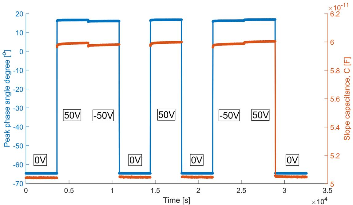
**Figure 9.18:** Stability measurement performed on an element from a 16+16 array with a *bottom frame* using the Agilent E4990A impedance analyser. The figure shows the peak phase angle in  $^{\circ}$  and the slope capacitance as a function of time at different bias voltages from  $-50\text{ V}$  to  $50\text{ V}$ . Stable values are seen throughout the 60 min steps.
