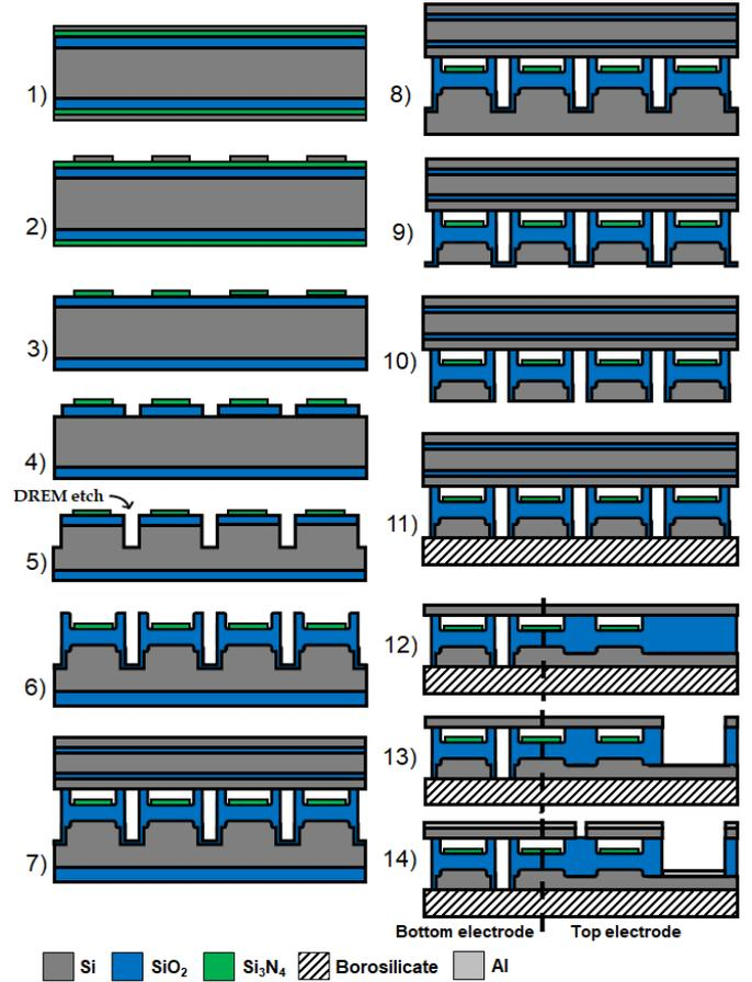
Figure 4. Fabrication process flow for the row-column CMUT array. The dashed line in drawings 12) through 14) represents a shift in perspective between a cross-section of the bottom electrode (to the left) and the top electrode (to the right).
