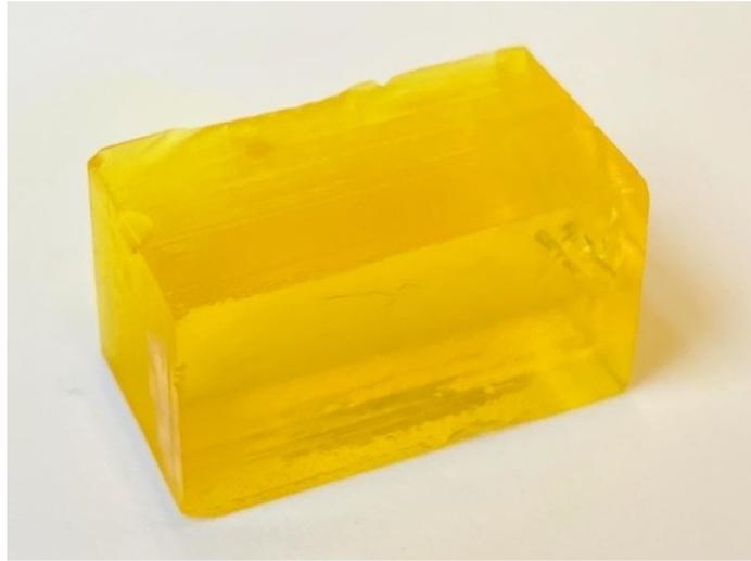
**Figure 6.35:** Stereolithography soft hydrogel phantom. The phantom dimensions are approximately  $1 \times 1 \times 2 \text{ cm}^3$  and has a grid of  $6 \times 4 \times 4$  isolated  $205 \times 205 \times 80 \mu\text{m}^3$  embedded cavities, spaced with a distance of 2.05 mm.
