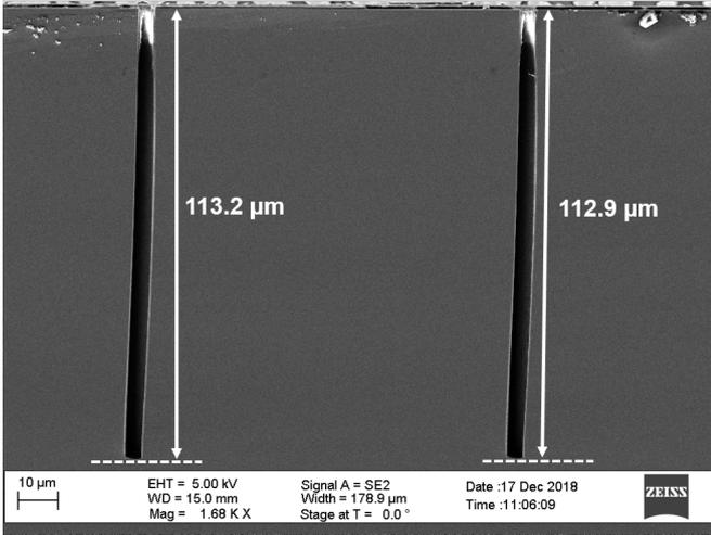
Fig. 3: Scanning electron microscope cross-sectional image of silicon wafer from step 1 in the fabrication process (Fig. 3). The etch depth of  $113\ \mu\text{m}$  is acquired after performing multiple deposit and removal cycles.
