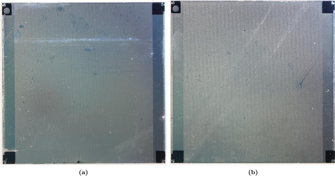
**Figure 5.5:** Photos of two finished TR2 chips, labelled (a) *TR2-O-1-Chip-1* and (b) *TR2-O-1-Chip-2* or simply *TR2-1* and *TR2-2*. The TR2-2 chip is the chip which will be further integrated in the probe for acoustical characterisation.
