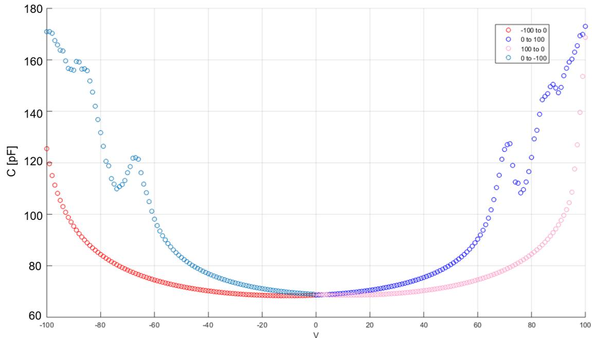
**Figure 9.2:** CV curve from a north-eastern long test element 190. This has been from  $-100$  V to  $100$  V. The voltage has been increased past with is estimated to be the pull-in voltage at around  $65$  V.
