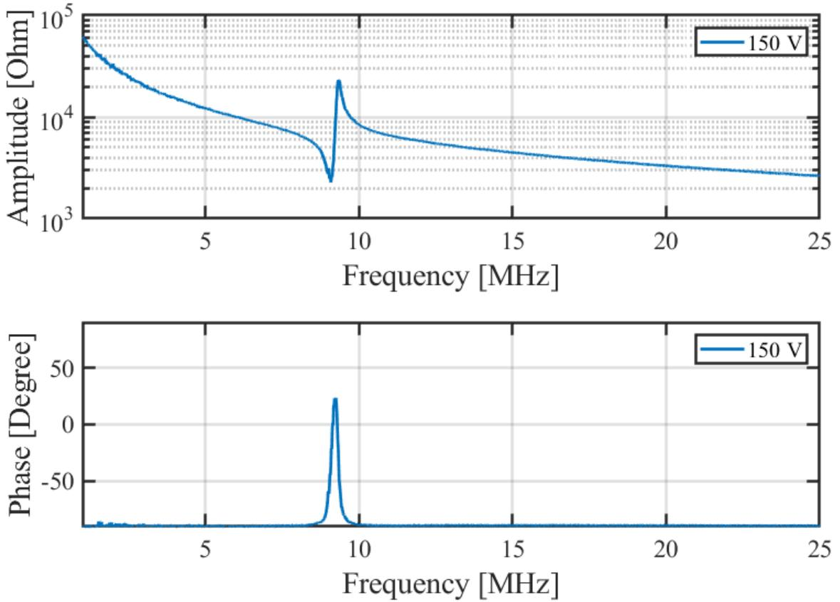
**Figure 3.6:** Plot of a typical Z-f impedance measurement on the Agilent E4990A, which can be measured from 20 Hz to 120 MHz. The magnitude of the impedance  $|Z|$  in  $[\Omega]$  and the phase angle  $\theta$  in  $[\circ]$  are plotted versus frequency from 1 MHz to 25 MHz.
