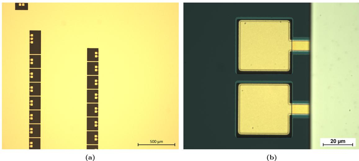
**Figure 8.11:** Microscope images showing the completed poly-Si etch with the opening to the bottom electrode pads. No nitride is present on top of the Au gold pads because of the openings made in the nitride on the PSOI wafer using the *Opening to bottom - SiN* photo mask.
