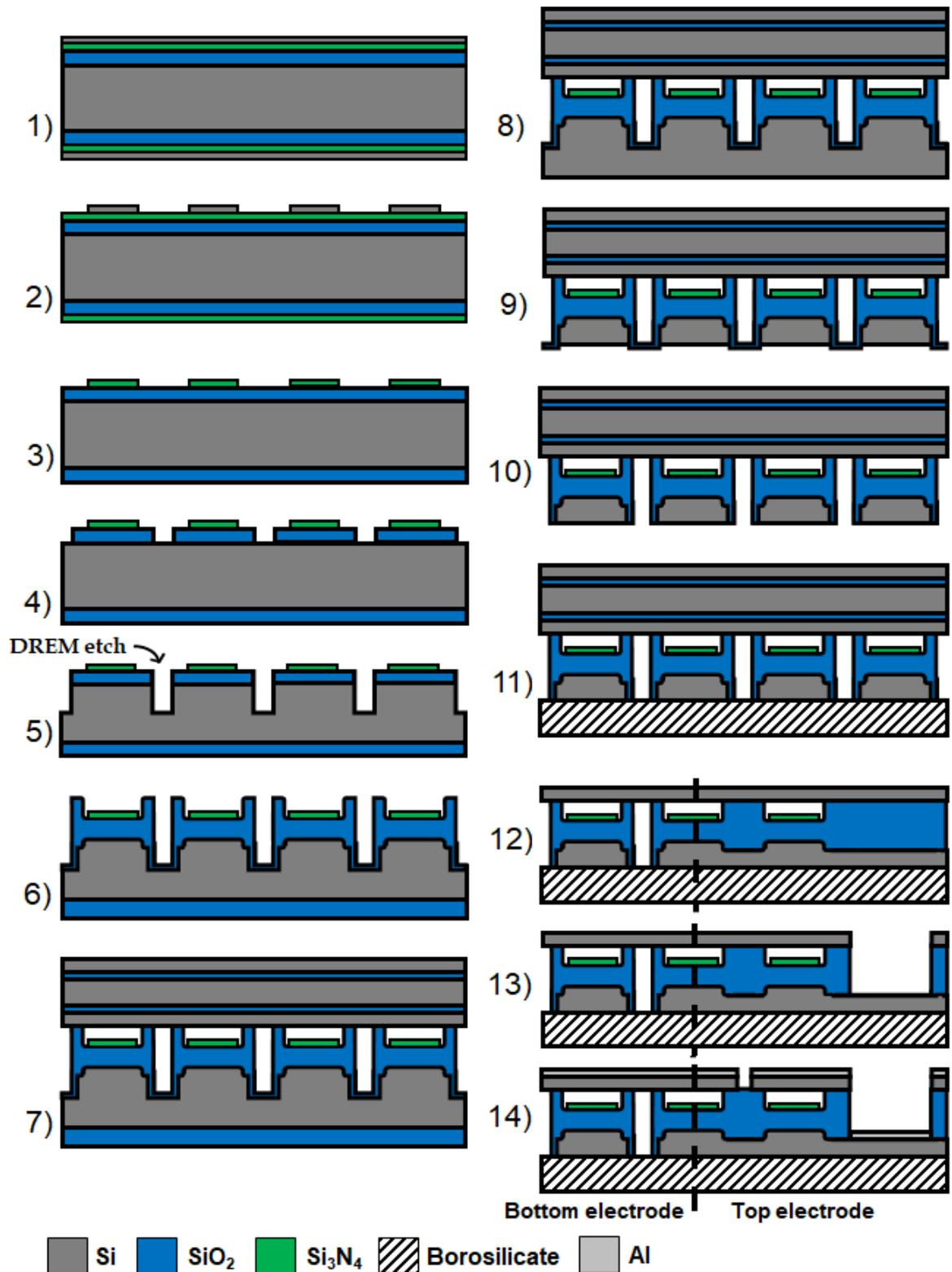
**Figure 5.1:** Fabrication process flow for the fusion and anodic row-column CMUT array. The dashed line in Fig. 12) through 14) represents a shift in perspective between a cross-section of the bottom electrode (to the left) and the top electrode (to the right). From [1].
