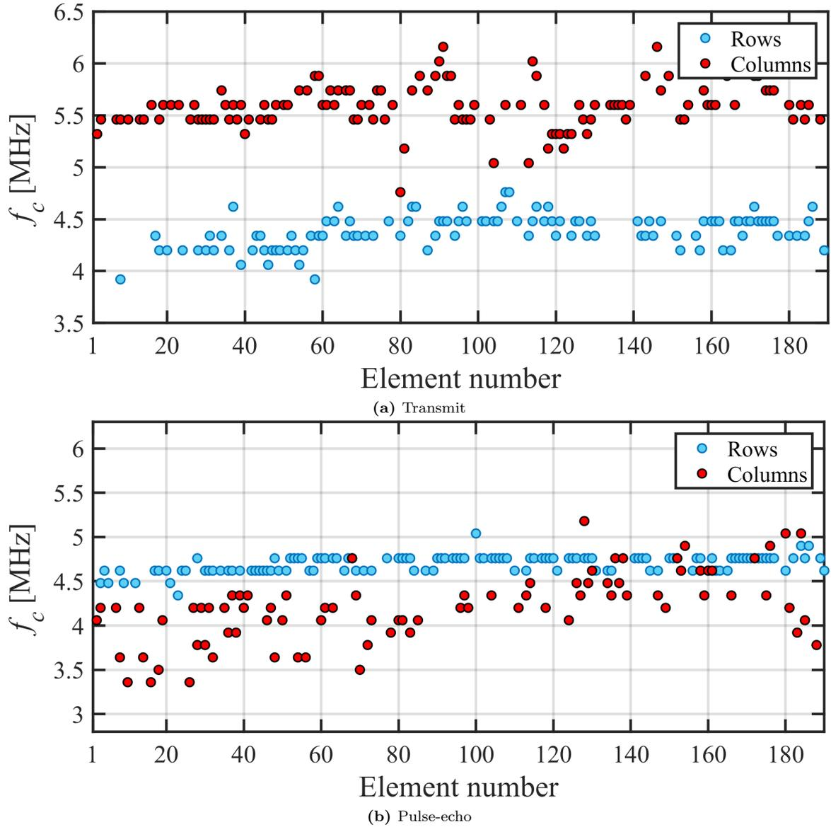
**Figure 6.24:** Extracted peak frequencies across the array for each element in transmit (a) and pulse-echo (b). The frequencies were found by using a peak-finding algorithm in MATLAB. The average center frequency of functional row and column elements in the probe is  $5.0 \pm 0.6$  MHz in transmit and  $4.5 \pm 0.4$  MHz in pulse-echo.
