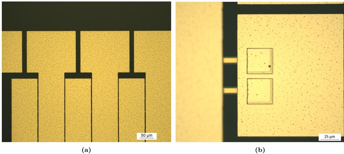
**Figure 8.15:** Microscope image of the top electrodes after the poly-Si etch in the ASE tool. (a) shows an overview of the separated top electrodes. (b) shows a bottom electrode pad separated from the top electrodes. The connecting leads covered by the nitride bridges are seen.
