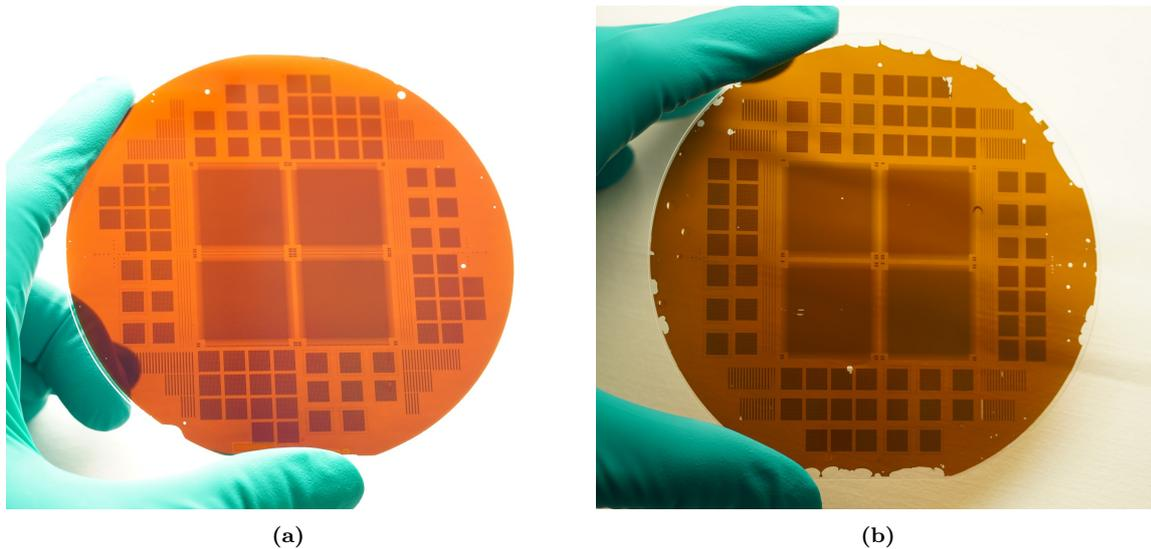
**Figure 8.9:** Photo of two wafers with a slightly different wafer layout and their handle layers removed. (a) can be seen to have very little voids not affecting any of the large arrays or smaller test arrays. (b) can be seen to have multiple small voids in the periphery and in the large center arrays, which will result in some unusable elements.
