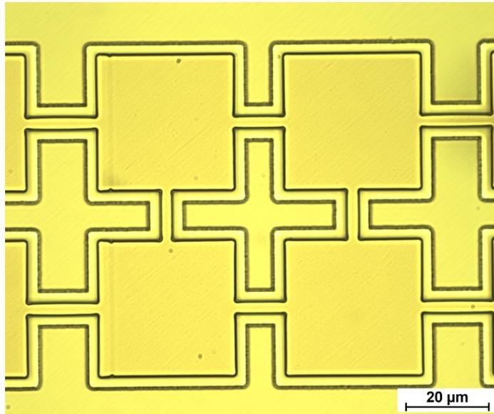
**Figure 8.3:** Microscope image of the *Bottom electrode* resist mask in the CMUT glass cavities on top of the Au electrode layer.
