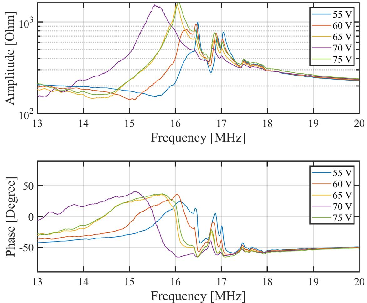
**Figure 9.16:** Impedance measurements of a long CMUT element corresponding to an element of the 190+190 RCA array. The impedance has been measured with a DC bias from 55 V to 75 V and a 50 mV AC. This demonstrates the CMUT element close to pull-in, estimated to be close to at 65 V. No clear indication of pull-in is seen, as the impedance amplitude peaks and phase angle peaks do not shift further down in frequency when the DC bias voltage is increased above 70 V.
