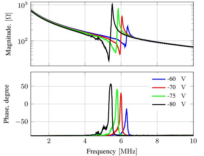
Fig. 6: Impedance measurements of the fabricated linear CMUT test array at four different DC biases with a  $50\ \text{mV}$  AC bias. The expected spring softening effect is observed for increased DC magnitude.
