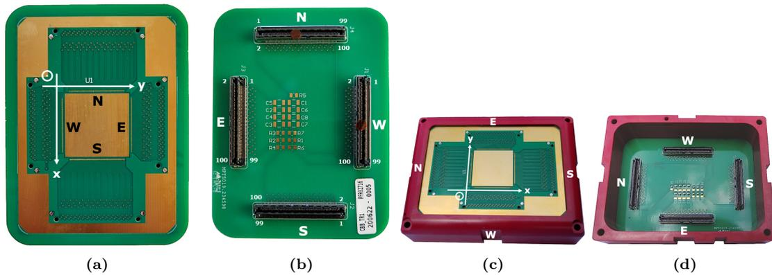
**Figure 9.19:** Photos [130] of: (a) Chip carrier board (CCB) and (b) CCB underside. (c) CCB in nose piece. (d) Backside of nose piece.
