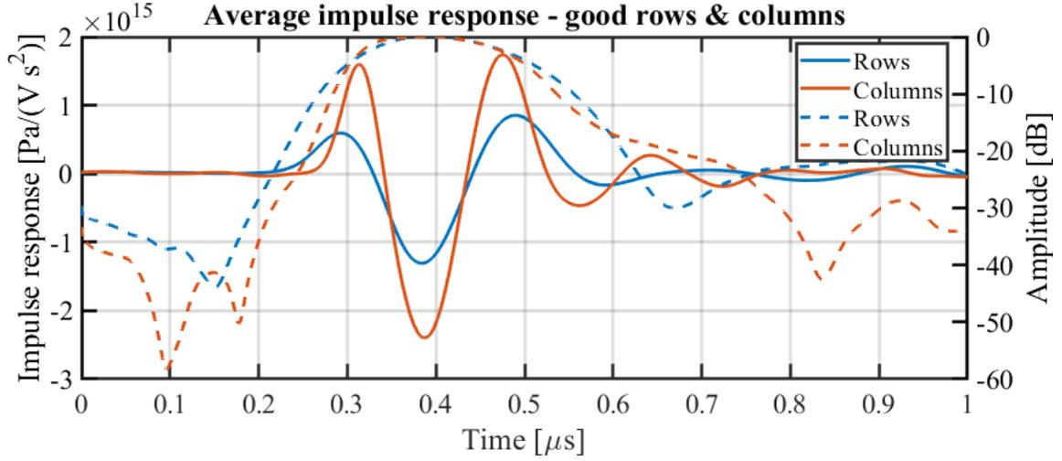
**Figure 6.17:** Average transmit impulse response (TX), as solid lines, and the normalised envelope (in dB), as dashed lines, of the functional row and column elements with amplitudes above  $1.1 \times 10^{15} \text{ Pa V}^{-1} \text{ s}^{-2}$ . From [1].
