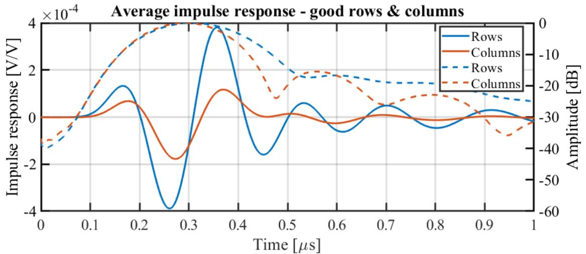
**Figure 6.21:** Average pulse-echo impulse response (PE), as solid lines, and the normalised envelope (in dB), as dashed lines, of the functional row and column elements with amplitudes above  $1.4 \times 10^{-4} \text{ V V}^{-1}$ . From [1].
