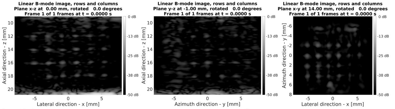
Figure 19. Point spread functions in three orthogonal planes obtained from a stereolithography 3D printed hydrogel phantom using the 190+190 transducer probe. The phantom has a grid of  $6 \times 4 \times 4$  isolated  $205 \times 205 \times 80 \mu\text{m}^3$  embedded cavities, which function as scattering point targets.
