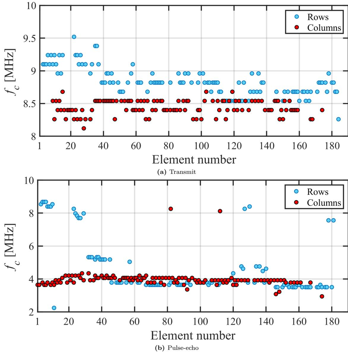
**Figure 9.39:** Extracted peak frequencies across the array for each element in transmit (a) and pulse-echo (b). The frequencies were found by using a peak-finding algorithm in MATLAB. The average center frequency of functional row and column elements in the probe is  $8.6 \pm 0.5$  MHz in transmit and  $4.3 \pm 1.3$  MHz in pulse-echo.
