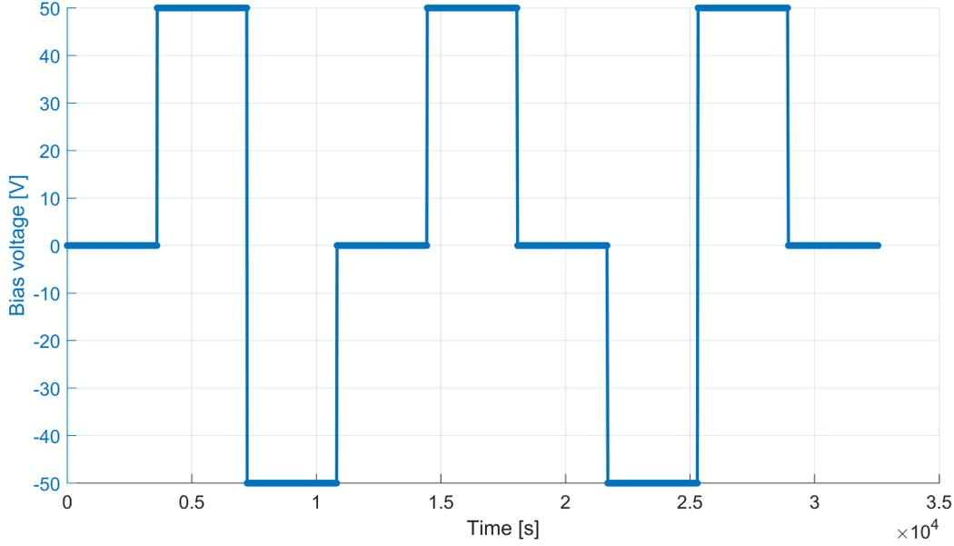
**Figure 3.9:** Bias voltage sequence used for testing the stability of the CMUT elements. The bias is held for an extended time period at each voltage step and the peak phase angle and capacitance is logged over time. The sequence depicted applies a  $\pm 50$  V bias held for 60 min at each step.
