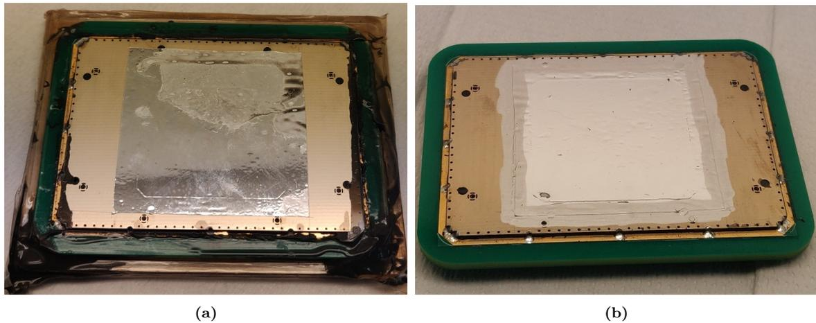
**Figure 9.26:** (a) Cutting the EMI shield to size and (b) gluing it to the frame with conducting glue (illustrated here with an Al film instead of the Torayfan PC3 film).
