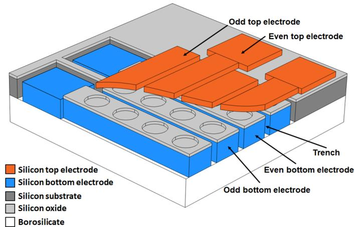
**Figure 1.5:** A 3D sketch of the corner of an RCA array made using the fusion-anodic double bonded method. The orthogonal blue bottom electrodes and orange top electrodes, made of silicon, are shown encapsulating the structured oxide layer with the circular CMUT cells. A wide trench is shown separating the bottom electrodes laterally, and a glass substrate (borosilicate) is shown bonded to the backside of the structure.
