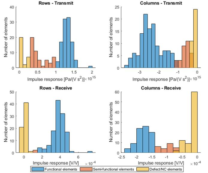
Figure 12. Histogram of impulse response of all row and column elements. The elements are grouped into three categories depending on their maximum impulse response values.
