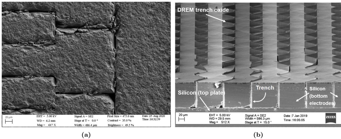
**Figure 5.3:** (a) Scanning electron microscope image of the backside of the silicon bottom electrodes after the lapping process occurring between step 8) and step 9). (b) Scanning electron microscope image of a test structure illustrating the cross-section of the backside of the wafer after step 9), before polishing. The exposed DREM trench oxide walls separating the bottom electrodes are clearly visible. This was also previously presented in [80].
