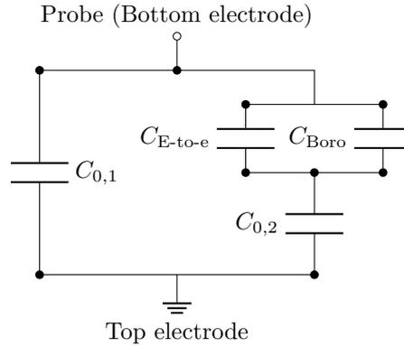
**Figure 6.26:** Circuit diagram of the neighbouring element coupling when probing column element 1, with  $C = C_{0,1}$  and the signal on the bottom electrode pad and ground on the top electrode. The parasitic capacitances  $C_{E-to-e}$  (short for element-to-element) and  $C_{Boro}$  (short for boro-fringe) as well as  $C_{0,2}$ , from the neighbouring element 2, couples into the probed element.
