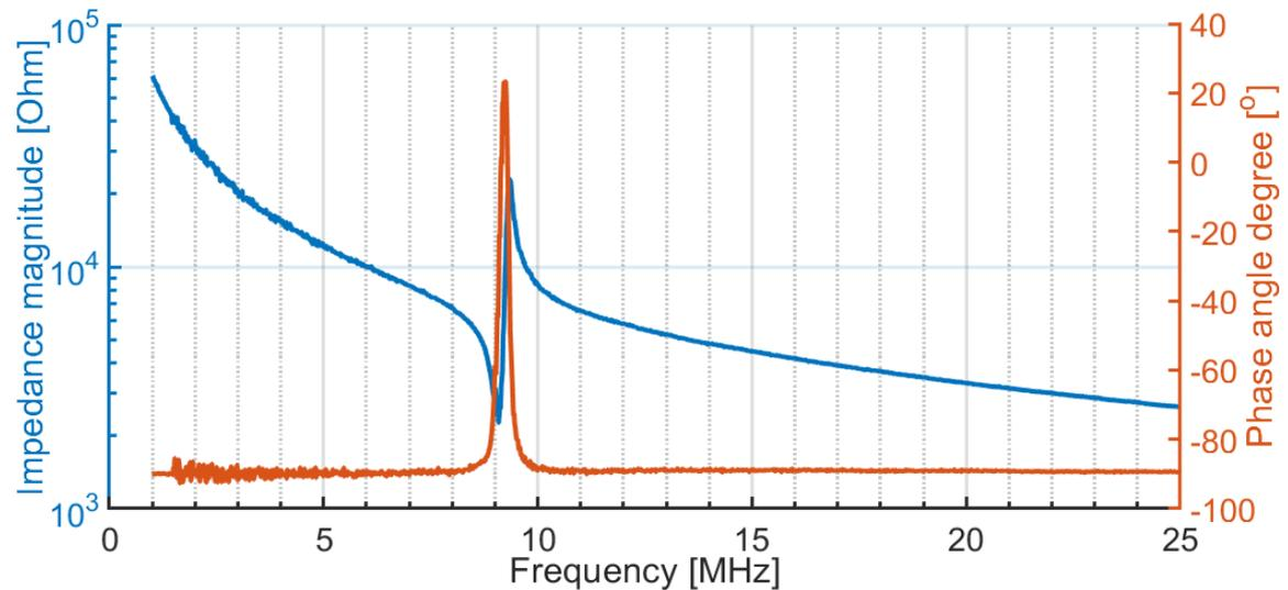
**Figure 6.5:** Impedance measurement of a CMUT test element at 150 V DC bias and 50 mV AC. The resonance and anti-resonance peaks are seen at 9.1 MHz and 9.3 MHz, respectively. Data is from a north-western placed test element on chip 1. From [1].
