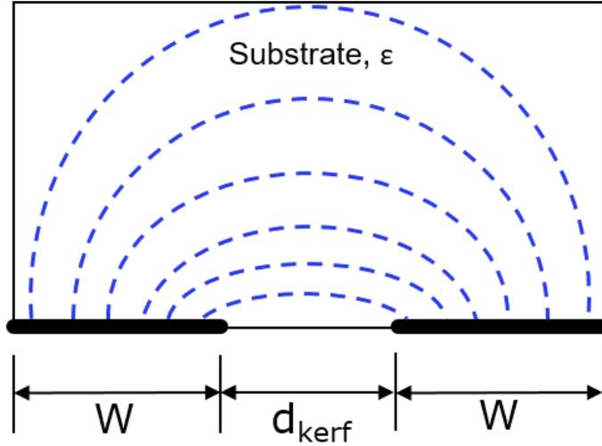
**Figure 6.25:** Sketch of the fringe electric field lines between the bottom of two electrodes with width,  $W$ , and the vacuum-filled kerf  $d_{\text{kerf}}$  separation. The structure is viewed upside down with the blue lines going through the substrate (indicated by the bounded box), with permittivity  $\epsilon$ , creating a parasitic capacitance.
