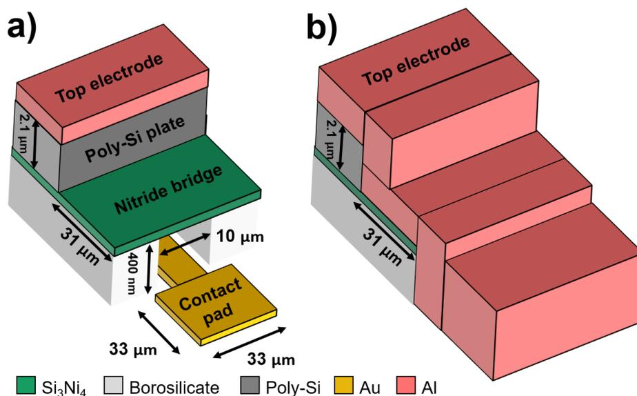
**Figure 8.12:** (a) Sketch of the borosilicate glass trench near the contact pad, covered by a silicon nitride bridge layer. A single 200 nm aluminium layer is on top of the plate. (b) the contact pad cavity plugged with 800 nm aluminium, which also seals the trench leading into the cells. The sketches are not to scale.
