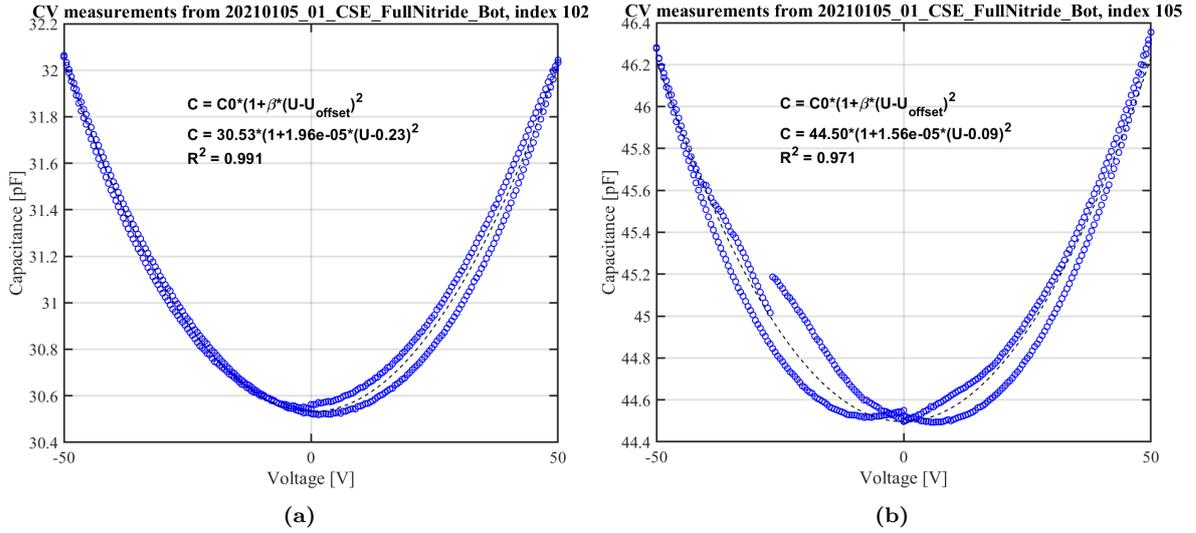
**Figure 9.8:** Data from CV tests for two bottom electrode neighbour to neighbour measurements. (a) measured between elements E102-E103 show hysteresis most prominently in the positive voltage sweep. This also affects the  $V_{\text{offset}}$  and is not reflected in the parabolic fit. (b) measured between elements E105-E106 shows hysteresis in both positive and negative voltage sweep, which is also not reflected in the fitted parameters but lowers the  $R^2$  value.
