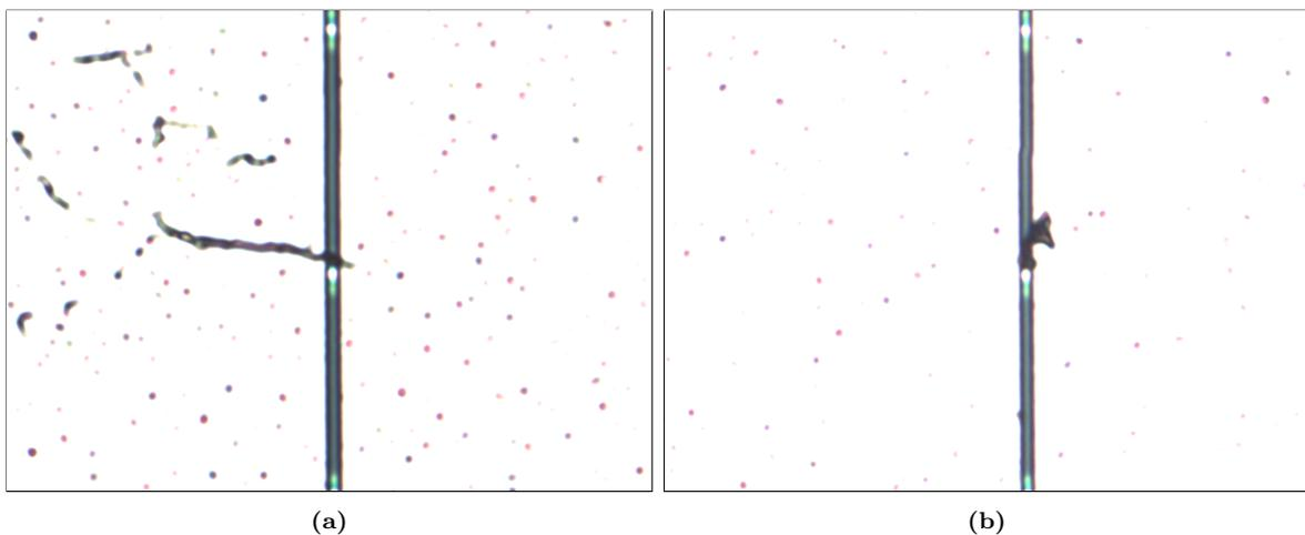
**Figure 9.7:** Microscope images of particles found on the wafer, which are believed to have acted as masks during the top electrode separation etch and are short-circuiting the two adjacent electrodes. (a) shows a particle strand between the shorted elements E9-E10 and similarly in (b) a particle is found in the kerf between the shorted elements E187-E188.
