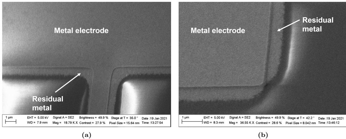
**Figure 8.5:** Images taken with a SEM of the bottom electrodes on test wafers without the glass cavities etched. A residual layer of gold is seen along the edges of the gold contact from the IBE etch.
