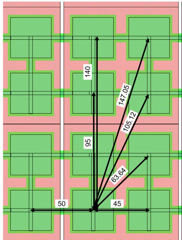
**Figure 7.3:** Seven nearest cell distances in the TH1 array design from L-Edit. The bottom electrodes and square cell cavities (green) are depicted going from left to right across the image and the top electrodes (peach red) in the orthogonal direction.
