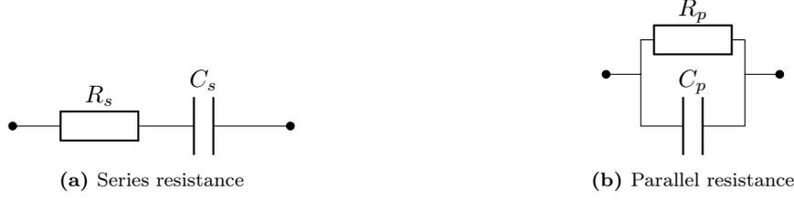
**Figure 3.4:** The measurement modes used by the analysers for expressing the impedance parameters and calculating the relevant  $C, L, R$  parameters. (a) shows the equivalent series mode circuit, with  $R_s$  and  $C_s$  being the series resistance and series capacitance. (b) shows the equivalent parallel mode circuit, with  $R_p$  and  $C_p$  being the parallel resistance and parallel capacitance.
