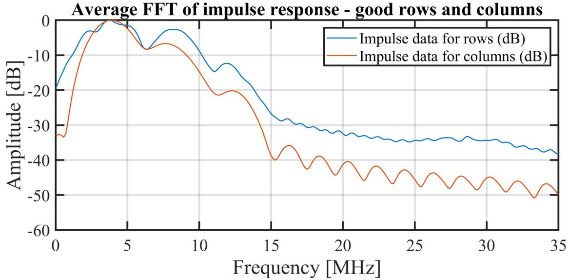
**Figure 9.37:** Average FFT spectra of the impulse response in pulse-echo (PE) of the functional row and column elements with impulse response amplitudes above  $1.4 \times 10^{-4} \text{ V V}^{-1}$ . The spectra for the rows and columns are normalised to the maximum of the average impulse responses with the values  $2.11 \times 10^{-4} \text{ V V}^{-1}$  and  $7.63 \times 10^{-5} \text{ V V}^{-1}$ , respectively.
