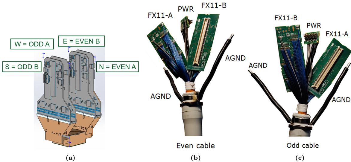
**Figure 6.12:** A 3D model view of the connected odd and even preamplifier board pairs illustrated in (a). Photos of the even (b) and odd (c) cables are shown with the two board connectors together with black grounding cables (AGND) and power leads (PWR).
