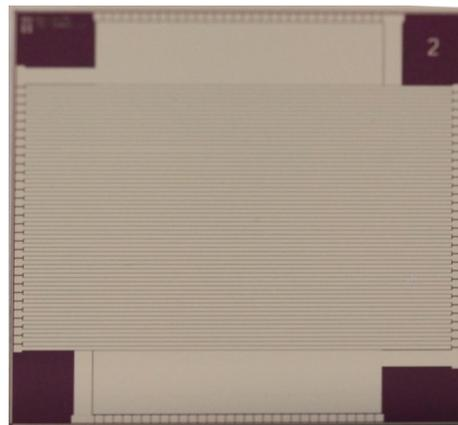
Fig. 1. Image of the 62+62 RCA CMUT chip
