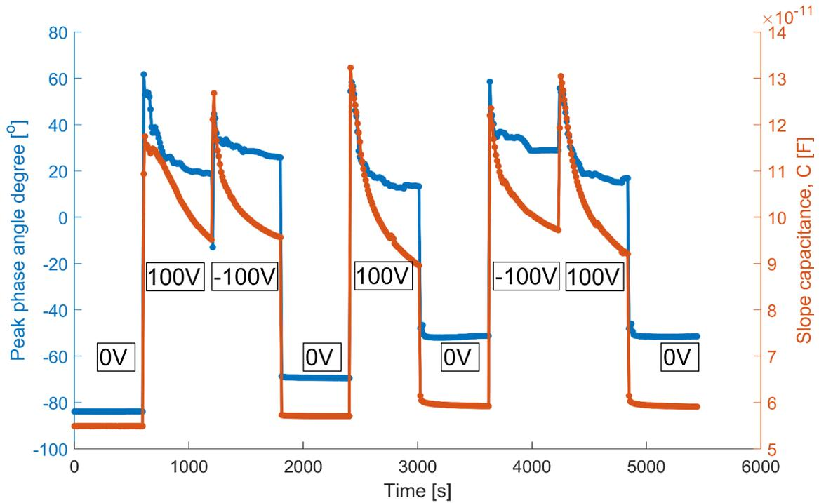
**Figure 9.17:** Stability measurement performed on a short 16 test element using the Agilent E4990A impedance analyser. The figure shows the peak phase angle in  $^{\circ}$  and the slope capacitance as a function of time at different bias voltages from  $-100\text{ V}$  to  $100\text{ V}$ . A clear decay of both values are seen for each of the 10 min steps.
