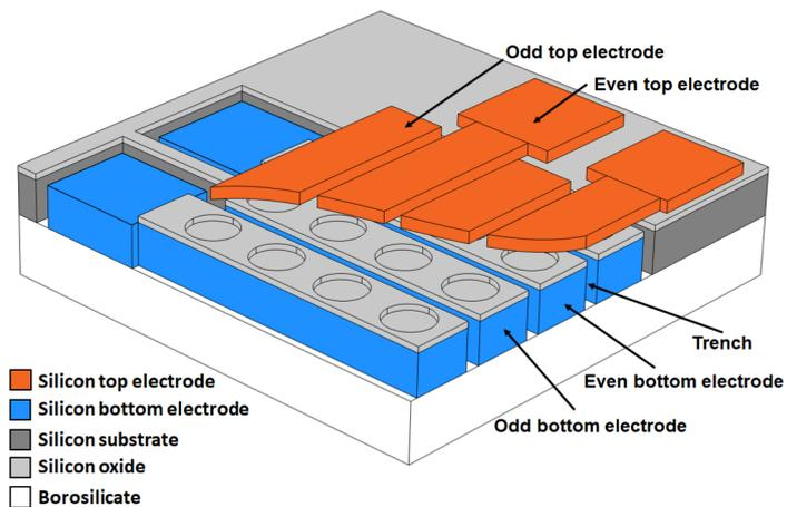
**Figure 4.3:** A 3D sketch of the corner of an RCA array with the same structure as the TR2 array. The orthogonal blue bottom electrodes and orange top electrodes, made of silicon, are shown encapsulating the structures oxide layer with the circular CMUT cells. A wide trench is shown separating the bottom electrodes laterally, and a glass substrate (borosilicate) is shown bonded to the backside of the structure.
