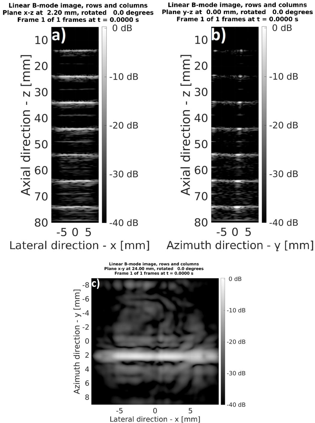
**Figure 6.37:** Imaging planes of a wire phantom obtained using the 190+190 TR2 transducer probe. The three different planes depict (a) the horizontal wires along in the x-direction (x-z plane), (b) two columns of wire cross-sections (y-z plane) and (c) the top of a single wire (x-y plane). From [1].
