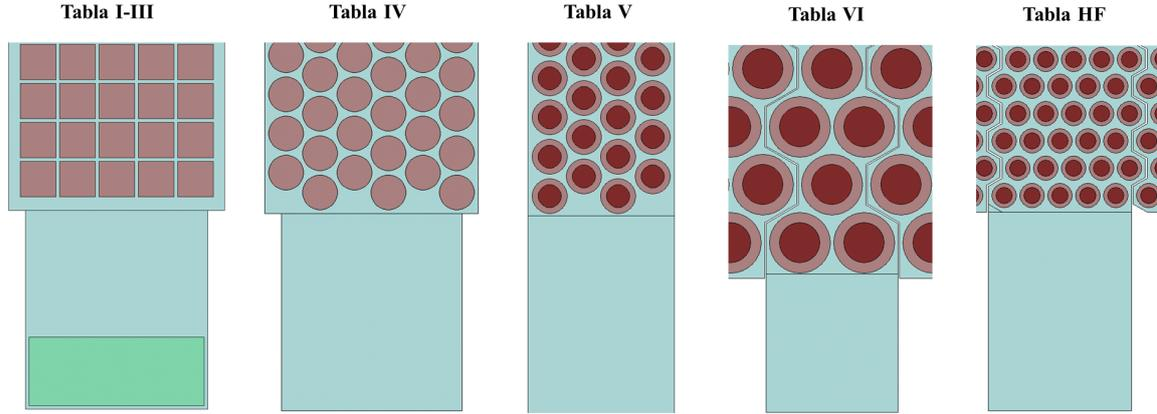
**Figure 2.2:** Illustrations of the mask layouts used for fabricating the linear Tabla CMUT arrays presented in [86]. Different cell packing schemes are demonstrated. For Tabla I-III a close packing optimal for square cells is used. Tabla IV and V used a type of HCP scheme. For Tabla VI and Tabla HF a type of interwoven HCP configuration is used where the elements overlap and the cell count either varies or is kept constant along the length of the element.
