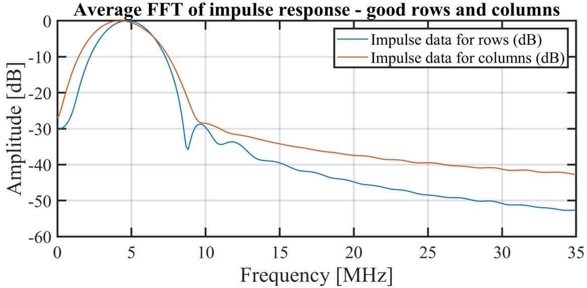
**Figure 6.22:** Average FFT spectra of the impulse response in pulse-echo (PE) of the functional row and column elements with impulse response amplitudes above  $1.4 \times 10^{-4} \text{ V V}^{-1}$ . The spectra for the rows and columns are normalised to the maximum of the average impulse responses with the values  $2.11 \times 10^{-4} \text{ V V}^{-1}$  and  $7.63 \times 10^{-5} \text{ V V}^{-1}$ , respectively. From [1].
