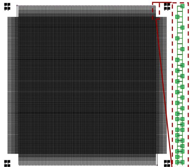
Figure 1. Design overview of the 192+192 row-column CMUT array. The integrated apodization scheme for one element is seen in the inset.
