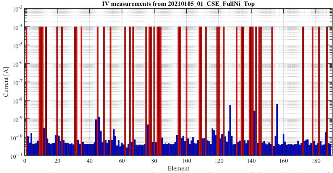
**Figure 9.5:** The maximum currents measured in the IV tests (on the y-axis) for each top element (on the x-axis) collected in a bar plot. A consistent low current from  $\sim 40$  pA to 110 pA, with a mean of  $163.6 \pm 626.9$  pA, is measured for the working elements (blue). Quite a few element are short-circuited above the current limit 100  $\mu$ A (red).
