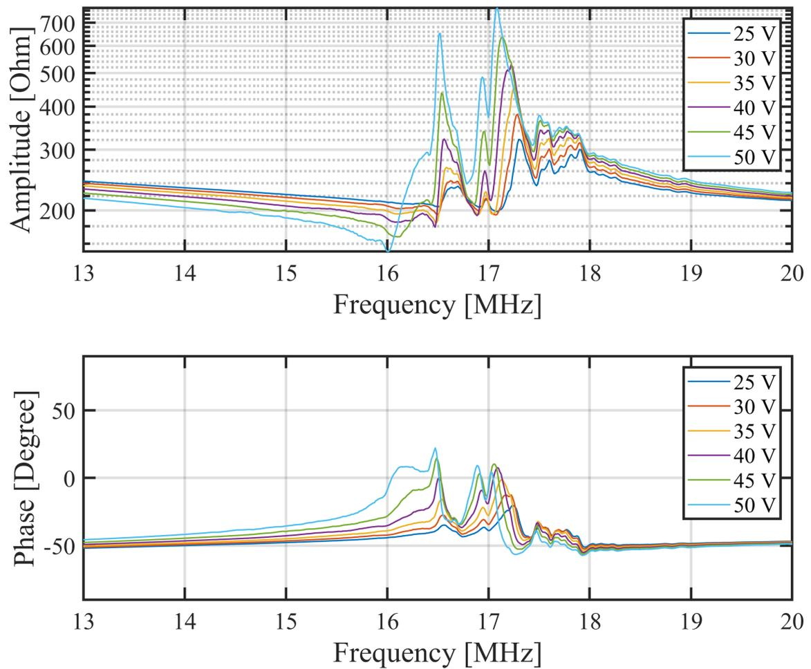
**Figure 9.15:** Impedance measurements of a long CMUT element corresponding to an element of the 190+190 RCA array. The impedance has been measured with a DC bias from 25 V to 50 V and a 50 mV AC. This demonstrates the CMUT element far from pull-in and at  $\approx 80\%$   $V_{\text{pull-in}}$  at 50 V.
