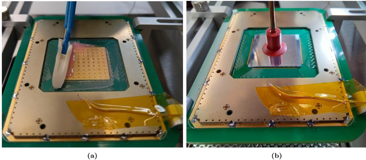
**Figure 9.21:** (a) Applying glue and (b) gluing the chip at an elevated temperature of 105 °C.
