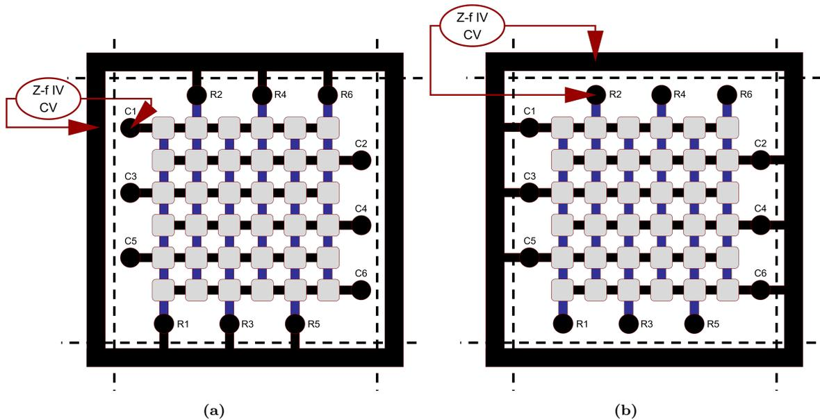
**Figure 3.1:** Sketch of two 6+6 row-column arrays with an extended electrode frame. This frame can be used to perform top to bottom electrode measurements, by connecting either all row elements (top electrodes) with a *top frame* (a) or by connecting all the column elements (bottom electrodes) with a *bottom frame* (b). The frames can be removed along the dotted lines in the chip dicing process. This makes it possible to use with an automated probe station with only two probes.
