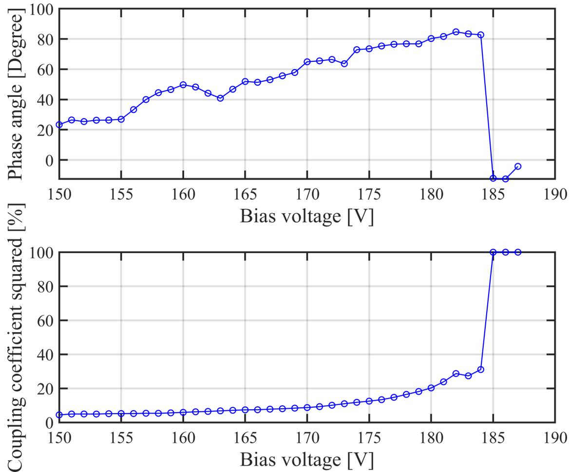
**Figure 6.4:** The maximum phase angle and coupling coefficient squared plotted as a function of DC bias voltage. The pull-in voltage is just at 184 V to 185 V as seen by the shift in phase angle and increase in coupling coefficient. Data is from a north-western placed test element on chip 1.
