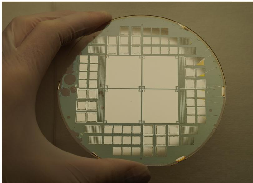
**Figure 8.16:** Photo of the finished TH1-A wafer after fabrication. Multiple voids in the left hand side, away from the 190+190 arrays are seen. In the south-east corner the been resist mask has burned slightly during the IBE etching process, which gives the metal a discolouration.
