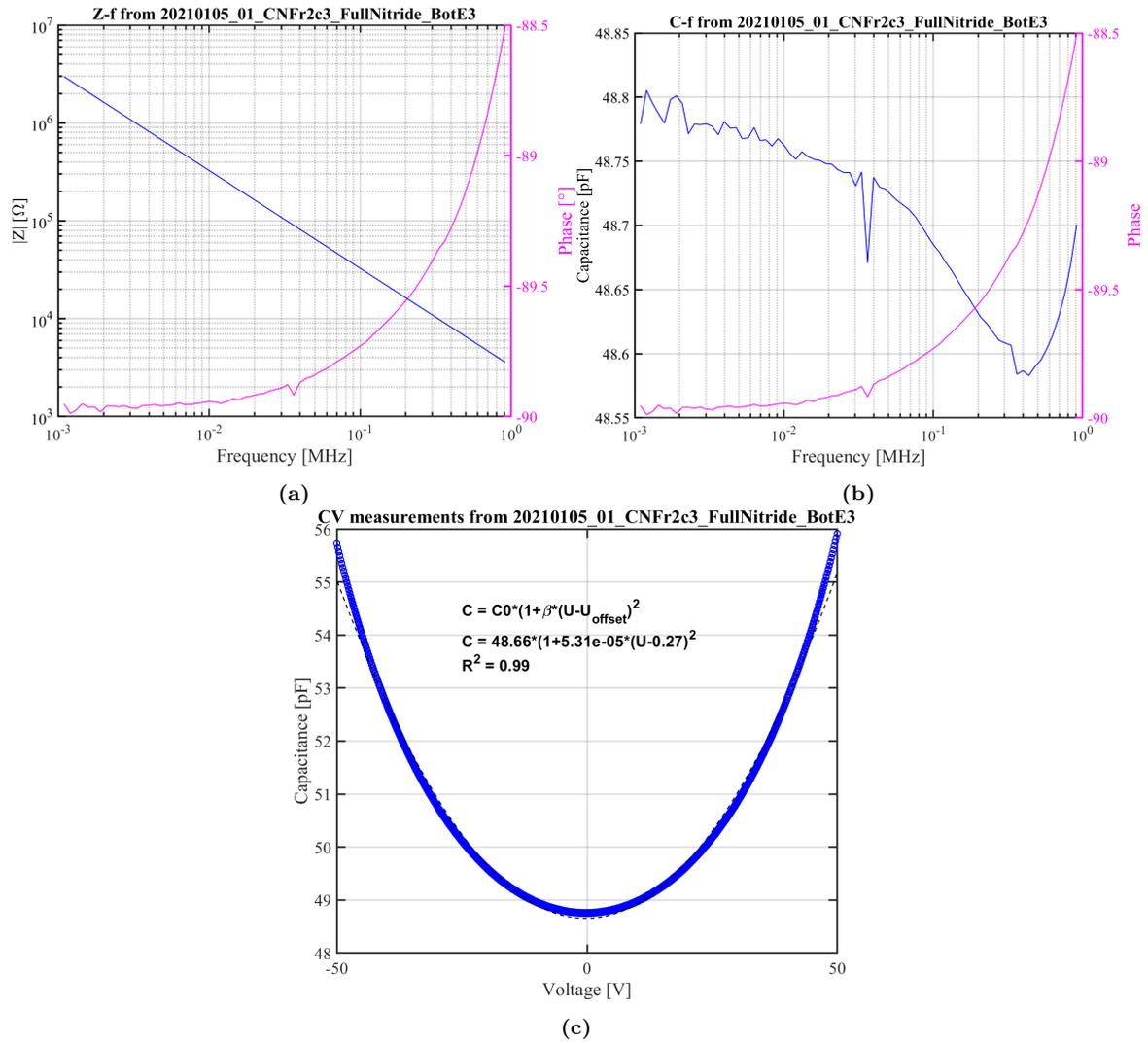
**Figure 9.3:** Northern 16+16 row-column array with a top frame. A bottom element has been probed to  $\pm 50$  V while the all the top electrodes are connected. A parabolic fit from Eq. 3.10 is included in the CV curve.
