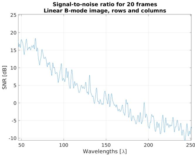
Figure 21. SNR of the 190+190 RCA probe for a tissue mimicking phantom with an acoustical attenuation of 0.5 dB/[MHz cm]. The penetration depth is roughly  $150 \lambda$  when the SNR reaches 0, corresponding to 3.6 cm as the wavelength in this phantom is 0.2375 mm when imaging with a frequency of 6.5 MHz.
