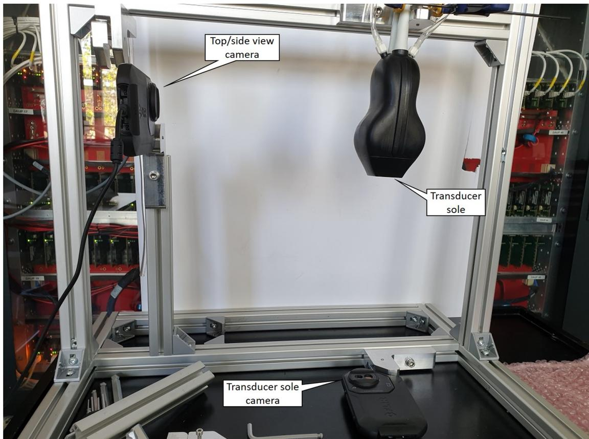
**Figure 6.31:** Thermal frame setup showing the fixed TR2 probe and two FLIR C2 thermal imaging system cameras; one camera is pointing at the sole surface and another at the side (or top part) of the assembled probe body.
