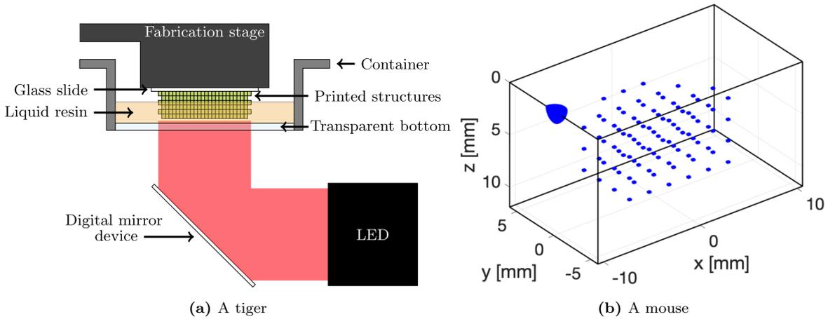
**Figure 6.34:** A 3D resin printer, shown in (a), is equipped with a 365 nm high power LED (LZ1-00UV00, Ledengin) source and a digital mirror device (DMD) used to selectively illuminated a thin layer of resin through the transparent bottom of the resin vat [125]. A 3D MATLAB design of a scatter phantom, shown in (b), with a grid of  $6 \times 4 \times 4$  isolated scatterer dots, spaced with a distance of 2.05 mm. This phantom has been designed by Martin Lind Ommen from this research group.
