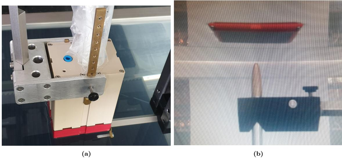
**Figure 9.30:** Photos of the acoustic measuring setup. (a) The prototype probe mounted to the AIMS III probe fixture with brass rails. (b) The hydrophone used during transmission measurements. This is mounted to a holder capable of moving in an x-y-z coordinate system.
