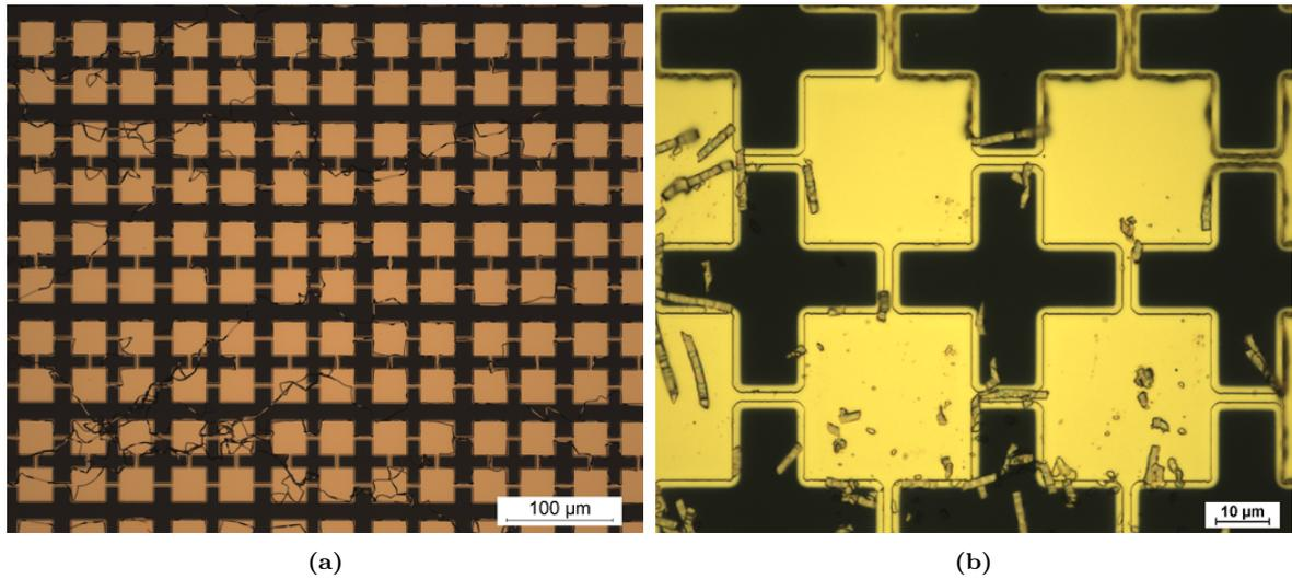
**Figure 8.17:** (a) shows gold ribbons from the IBE etching process adhering to the wafer surface after a wet resist strip. (b) shows the gold ribbons breaking of the electrodes and falling onto the surface after a resist strip using plasma ashing.
