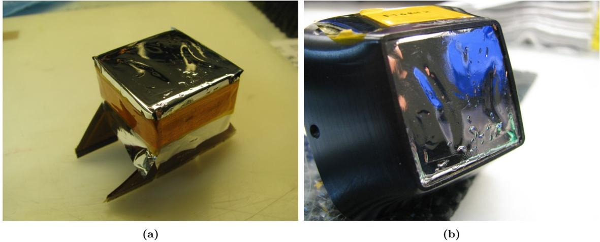
**Figure 6.10:** The photos show the assembly in progress just after the application of the first RTV silicone layer on the chip and the applied aluminised polymer grounding shield (a) and the subsequent mounting of the array in the nose piece (b).
