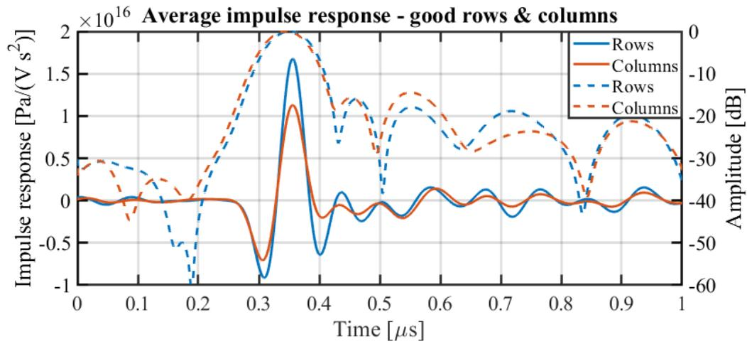
**Figure 9.31:** Average transmit impulse response in transmit (TX), as solid lines, and the normalised envelope (in dB), as dashed lines, of the functional row and column elements with amplitudes above  $6.94 \times 10^{15} \text{ Pa V}^{-1} \text{ s}^{-2}$  for rows and above  $5.18 \times 10^{15} \text{ Pa V}^{-1} \text{ s}^{-2}$  for columns.
