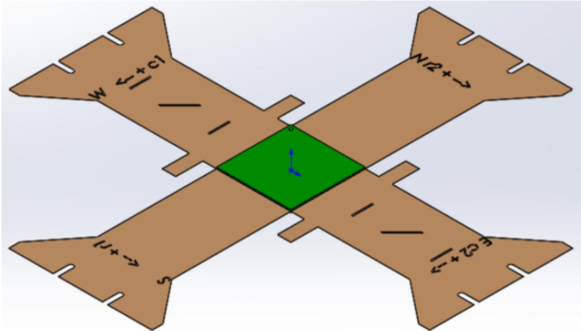
**Figure 6.6:** 3D drawing of the rigid-flexible PCB. The green center square of the rigid PCB part where the chip is mounted with glue. The dot in the north-western corner of the chip is aligned with the dot on the PCB. On each section of the flexible connectors are indicated the orientation of the chip of the starting row or column number for that connector, e.g. "N r2+>" indicating the north side of the chip starting with the even row element r2, counting up towards the right.
