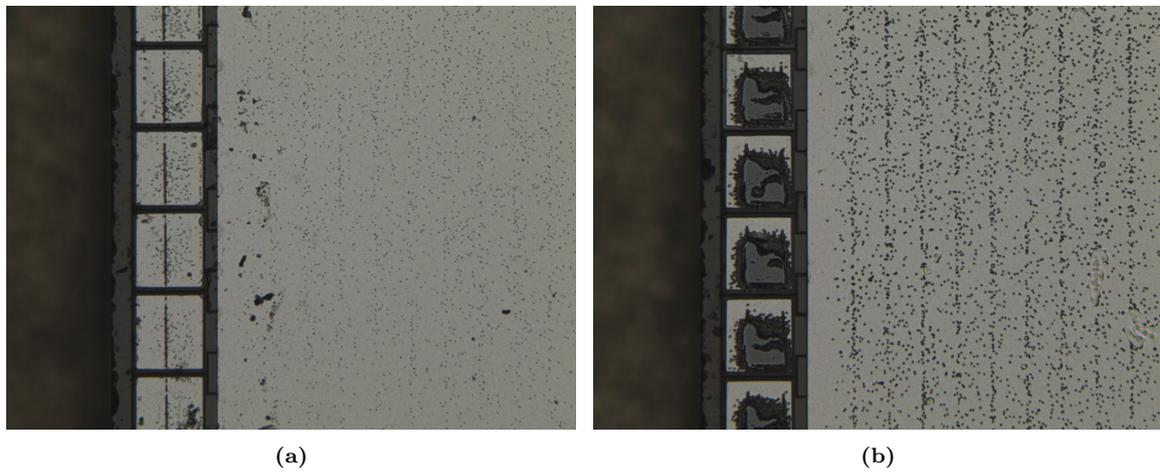
**Figure 5.7:** Images taken of the *TR2-2* chip after fabrication and dicing. In (a) a small amount of damage to the bottom electrode metal is seen. In (b) severe electrode damage is seen, presumably as a result of the incomplete bottom electrode access etch caused by the presence of the sulphur compound.
