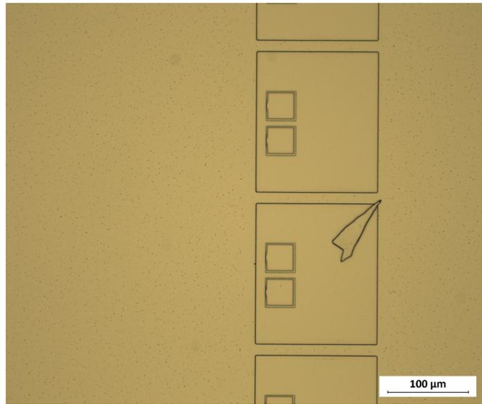
**Figure 8.13:** Microscope image of the Al-plugged contact pads and the larger rectangular electrode before top electrode separation. A poly-Si flake from the plate is seen partially covering one of the large contact pads.
