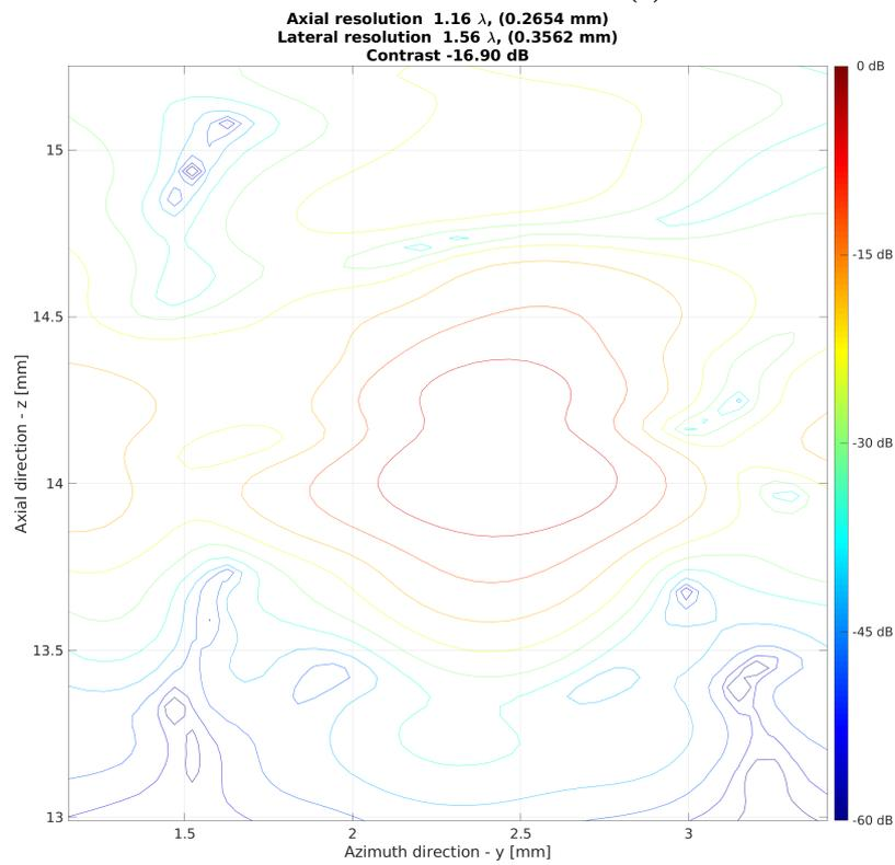
**Figure 6.38:** Point spread functions of the scatter phantom in the x-z plane (a) and of the wire phantom in the y-z plane (b).
