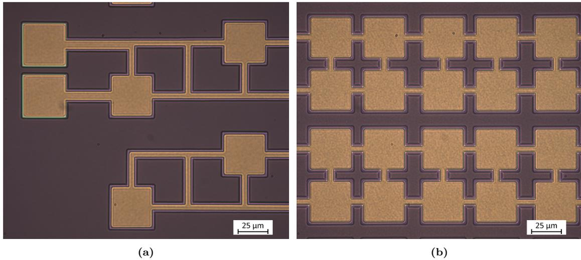
**Figure 8.7:** Microscope image of the metal bottom electrodes inside the glass cavities. The image is taken from the backside of the bonded wafer through the 500  $\mu\text{m}$  thick glass substrate.
