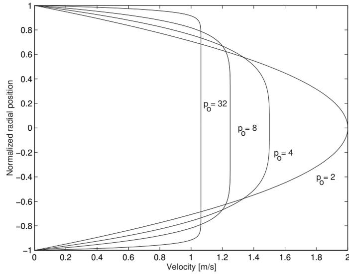
Figure 3.9: Velocity profiles for different values of  $p_o$ . The spatial mean velocity is the same for all profiles.
