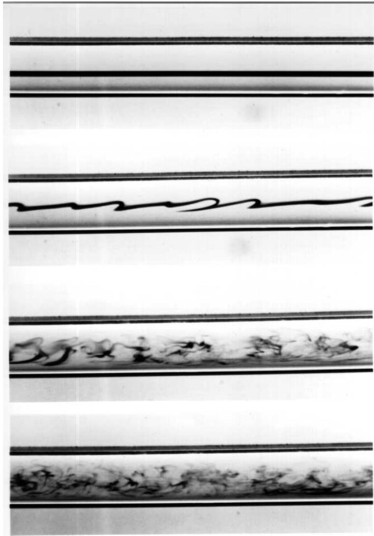
Figure 3.7: Photo of a dye injected into a tube with flowing water. The images are taken of the original apparatus as used by Reynolds in 1883 (courtesy of C. Lowe, Manchester School of Engineering).
