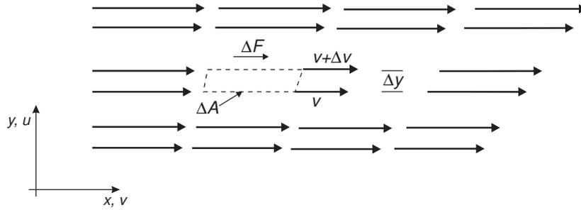
Figure 3.5: Force on small fluid volume in a rigid tube enclosing a steady flow.
