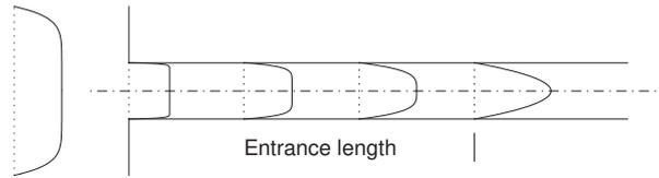
Figure 3.8: Development of a steady-state parabolic velocity profile at the entrance to a tube.
