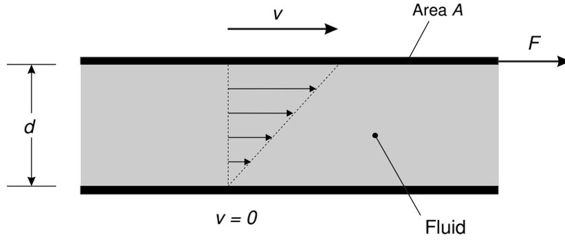
Figure 3.4: Viscous drag between two parallel plates.
