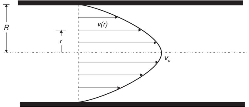
Figure 3.6: Laminar flow in a long, rigid tube.
