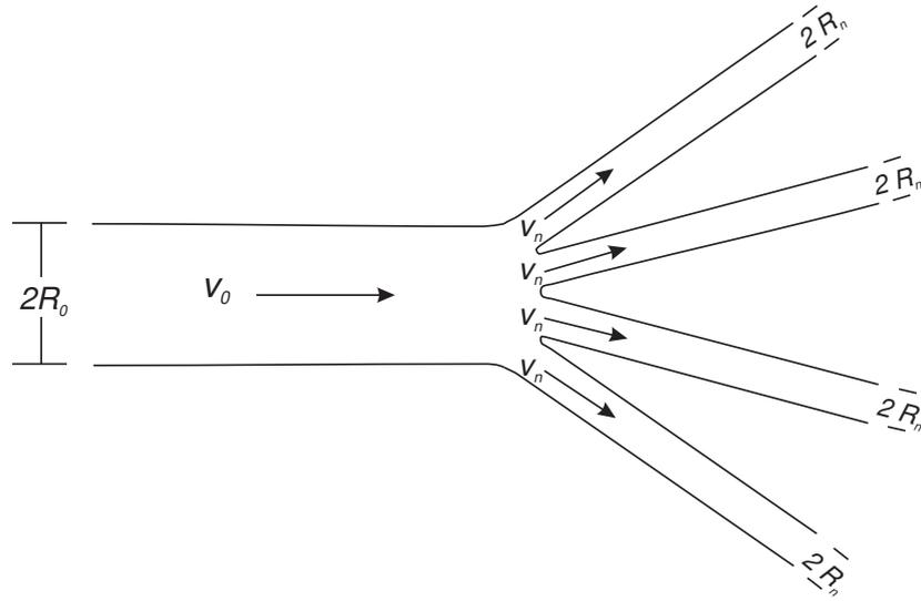
Figure 3.14: Steady flow in a rigid tube supplying  $n$  smaller tubes.
