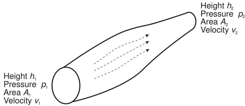
Figure 3.3: Flow in a narrowing tube.
