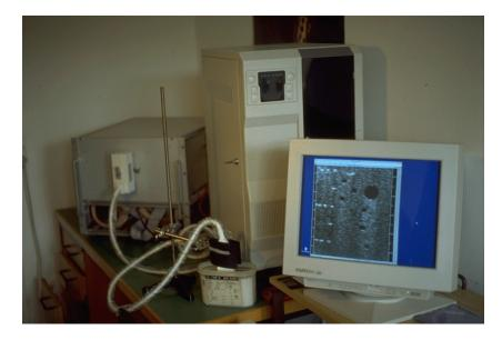
Figure J.1: The hardware of the XTRA system. The 19" rack is seen on the left, the control PC is in the middle, and the screen showing a conventional image of tissue mimicking cyst and a wire phantom is seen on the right. (Picture taken from [39])
