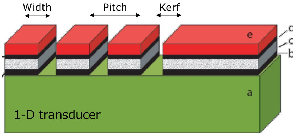
$$\text{Width} = \text{pitch} - \text{kerf}$$
