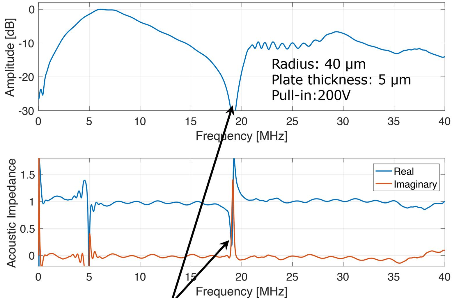
Frequency dip = (Speed of sound) / (cell pitch) =  $\sim 18$  MHz
