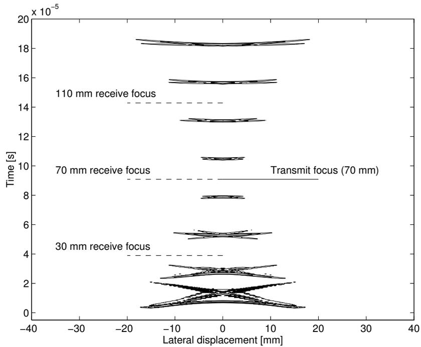
Figure 3.7: Point spread functions for different positions in a B-mode image. Onehundredtwentyeight  $0.2 \times 5$  mm elements are used for generating and receiving the pulsed field. Three different receive foci are used. The contours shown are from 0 to -24 dB in steps of 6 dB relative to the maximum at the particular field point (from [9], Copyright Cambridge University Press).
