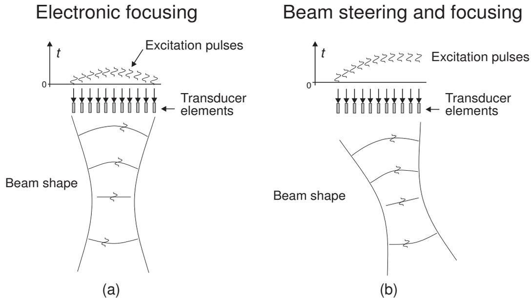
Figure 3.9: Electronic focusing and steering of an ultrasound beam.
