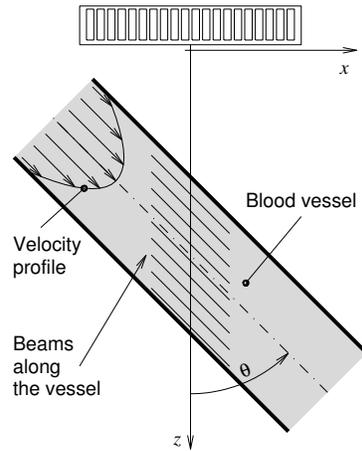
Figure 5.17: Directional beamforming along the flow lines (from [96]).
