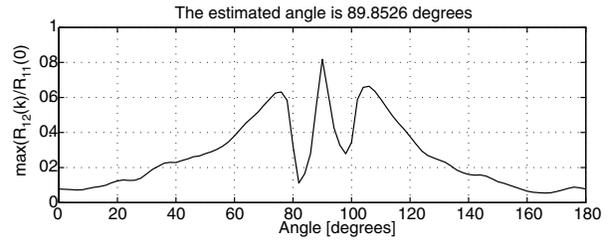
Fig. 11. Normalized maximum correlation as a function of beam formation angle.
