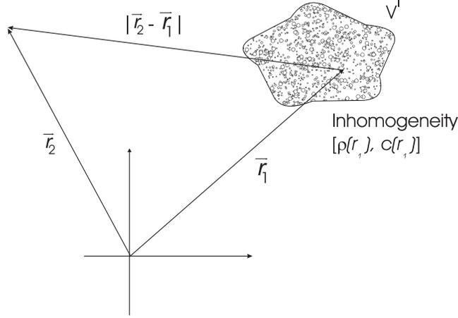
Figure 2.16: Coordinate system for calculating the scattered field
