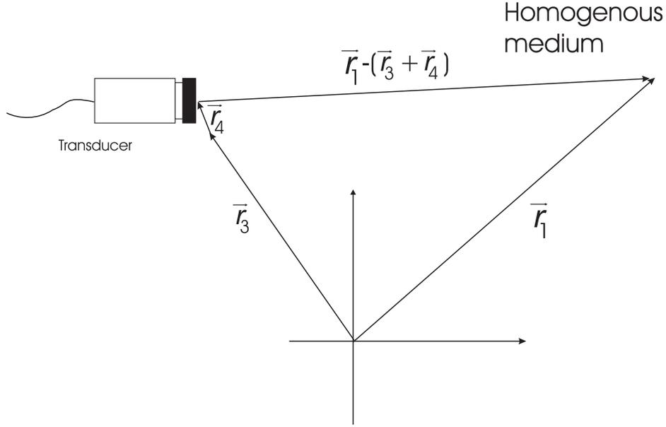
Figure 2.17: Coordinate system for calculating the incident field.
