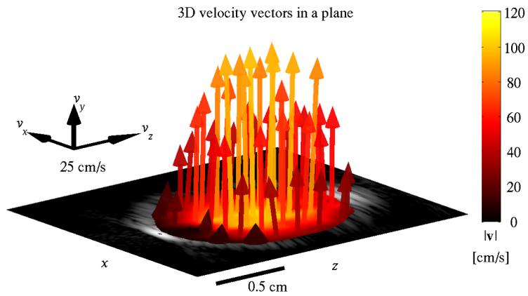
Figure 5.13: 3D vector velocity image for a parabolic, stationary flow (from [79]).
