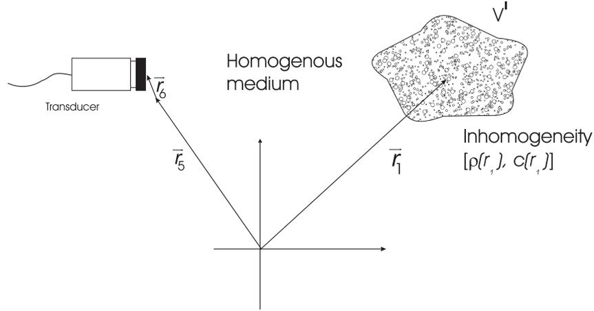
Figure 2.18: Coordinate system for calculating the received signal.
