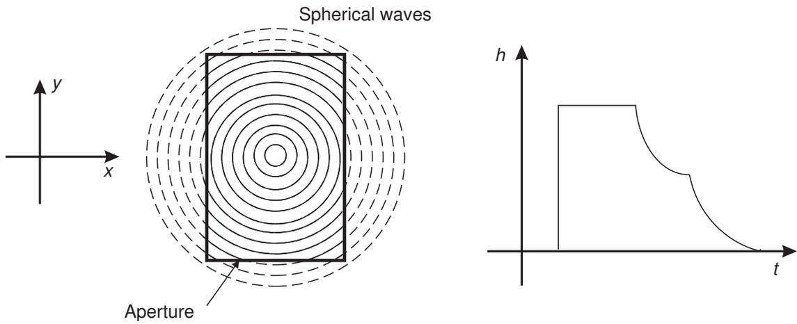
Figure 2.13: Schematic diagram of field from rectangular element.
