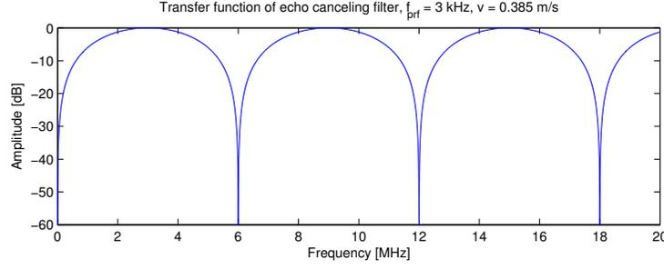
Figure 5.6: Transfer function of echo canceling filter.
