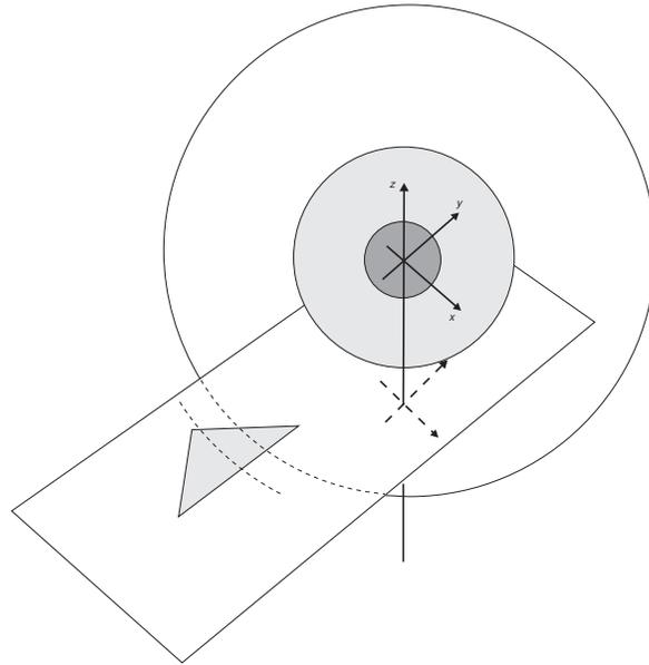
Figure 2.5: Emission of a spherical wave from the field point and its intersection of the aperture.
