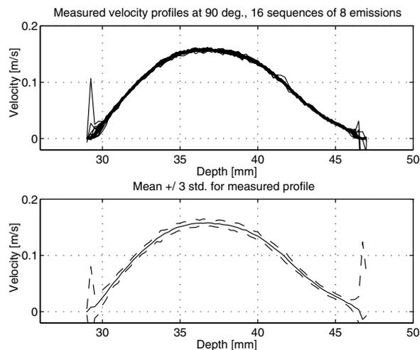
Fig. 8. Estimated profiles from the flow rig at a  $90^\circ$  flow angle. The top graph shows 20 independent profiles estimated and the bottom graph shows the mean profile (solid line)  $\pm 3$  standard deviations (dashed lines). From [38].
