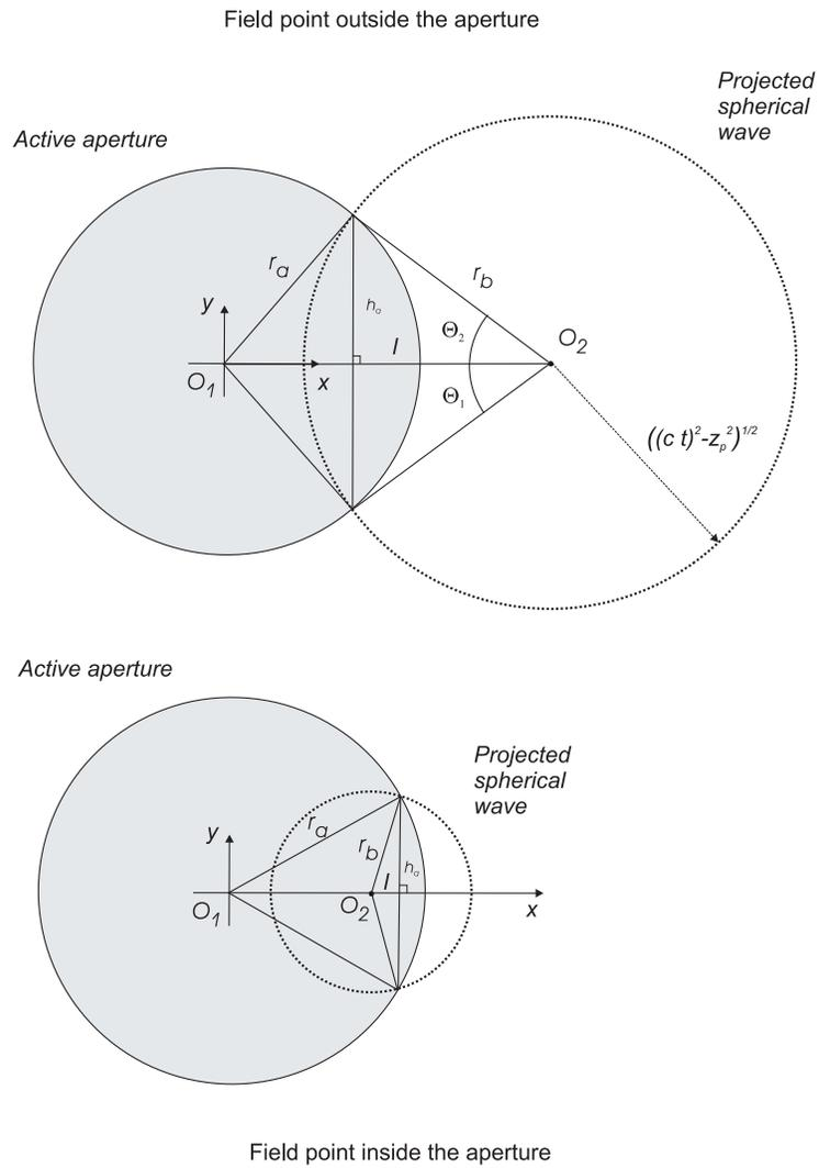
Figure 2.10: Geometry for determining intersections between circles. The top graph shows the geometry when the field point denoted by  $O_2$  is outside the aperture, and the bottom graph when it is inside.
