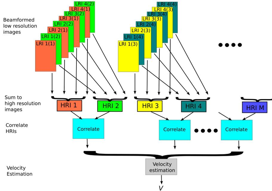
Fig. 4. Interleaved SA sequence where LRIs are repeated to minimize the distance between HRIs. The same colored LRIs are summed to yield one HRI. The effective  $f_{\text{prf,eff}}$  is equal to the highest possible value due to the interleaving. Correlations in the blue boxes yield the same correlation function, which are then averaged to improve precision.
