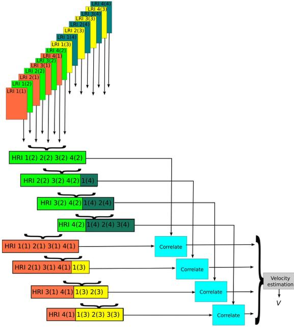
Fig. 5. Processing scheme for recursive SAF, where a new HRI is created after each pulse emission. *HRI 2(2) 3(2) 4(2) 1(4)* indicates which set of emission are used. The first number is the emission (virtual source) and the second number in parentheses is the sequence number used. Therefore, 3(2) is emission number 3 in the second sequence indicated by the light green color.
