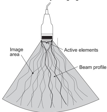
Figure 3.11: Phased array transducer for obtaining a polar cross-sectional image using a transducer with a small foot-print.
