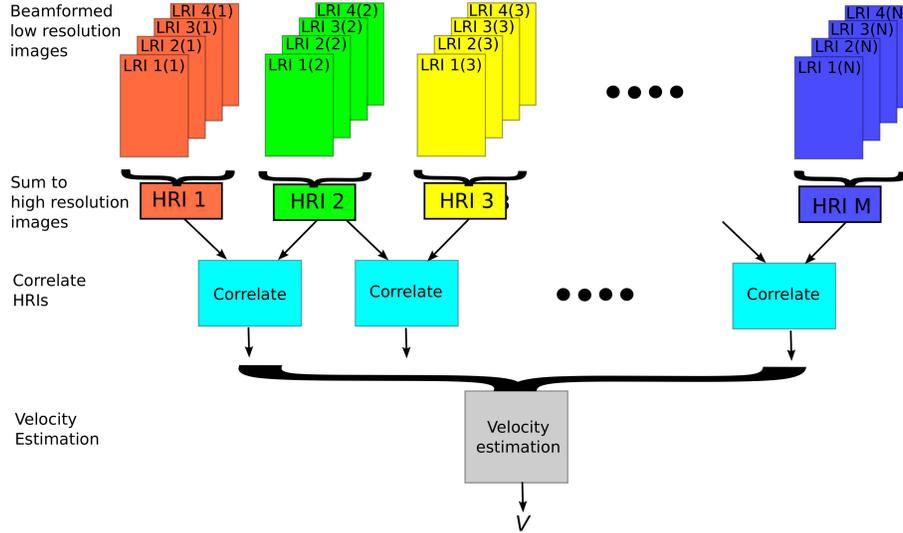
Fig. 3. Traditional SA sequence for velocity estimation. HRIs are created in blocks making the effective  $f_{\text{prf,eff}}$  low. LRI 1(2) denotes LRI for emission 1 in high-resolution sequence 2 (first emission in the green block).
