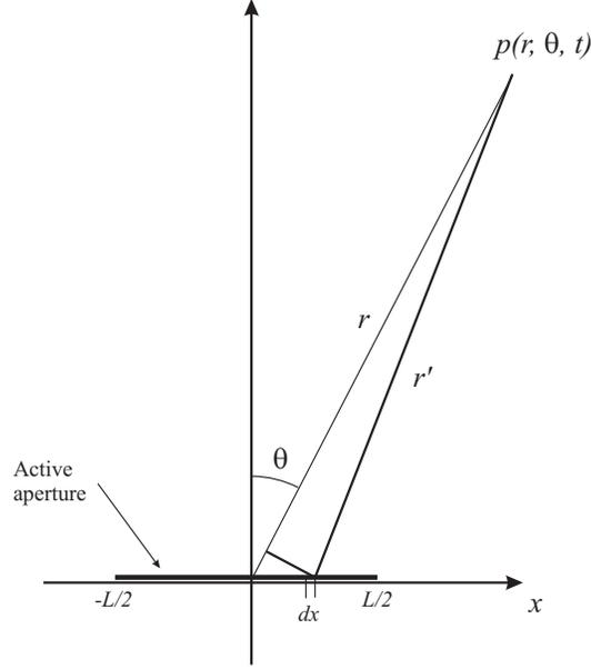
Figure 3.1: Geometry for line aperture.
