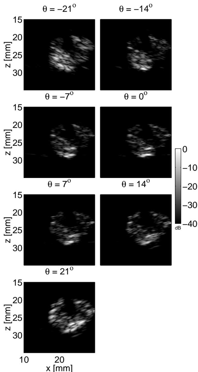
**Figure 6** The seven single-angle images used to create the compound image in Figure 5a.
