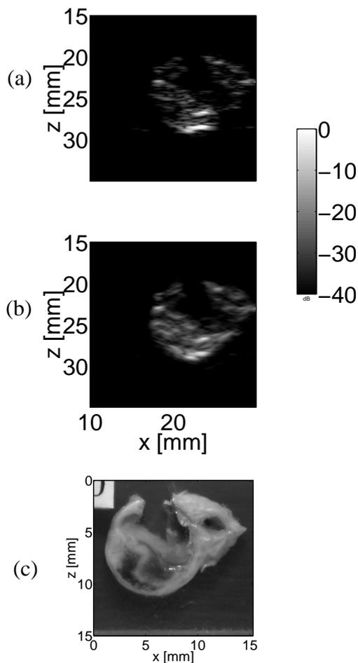
**Figure 5** (a) conventional and (b) compound cross-sectional images of atherosclerotic plaque. (c) macroscopic photograph taken at the same plane as the ultrasound image. The photograph was taken during slicing of the plaque.
