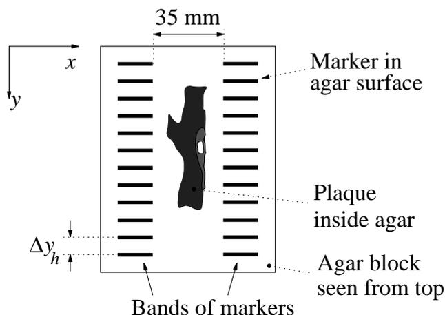
**Figure 4** Illustration of the components of the agar block, as seen from the top (= as seen from the transducer). The plaque is completely inside agar, while the agar markers are located on the top of the block. The drawing is not to scale.
