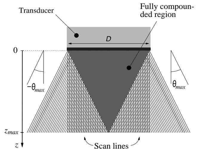
**Figure 1** Illustration of scan lines and angles for the recording of three single-angle images used in creating the multi-angle compound image.
